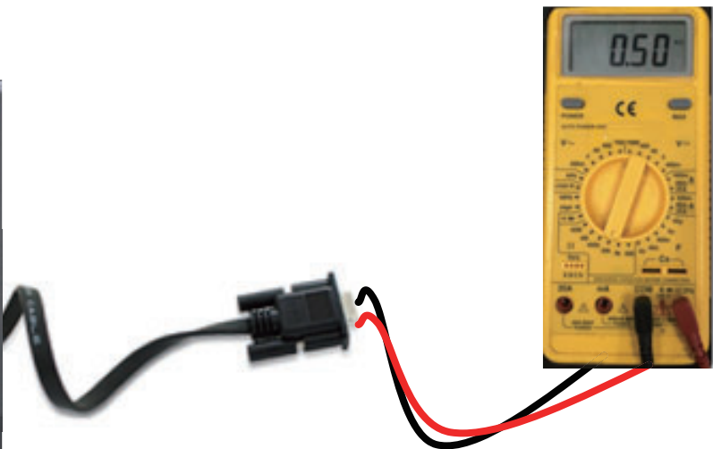
Three meter resistance measurement NTC's resistance is 0.50 K \Omega
