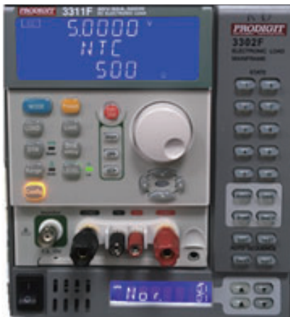
3302F/G frame with NTC module set NTC resistance is 500 K \Omega
