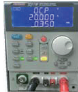
Figure 12 3311F/G with BMS for over current discharge test result ( single pulse )
