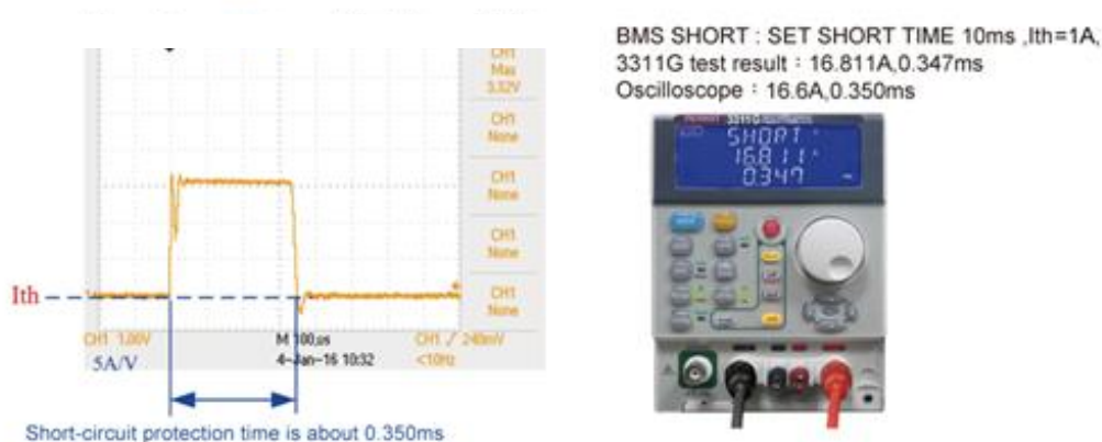
Figure 2.4 4000mAh Power Bank Actual Short Circuit Test Waveform
