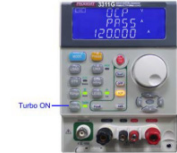
3311G Turbo mode ON OCP test result screen
