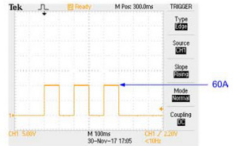
Turbo : OFF, Fuse ON, CC pulse 60A, 100mS, repeat 3 cycles real test waveform
