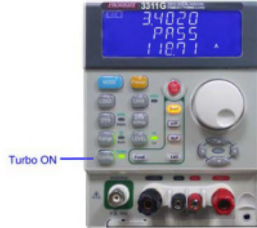
3311G Turbo mode ON Short test result screen
