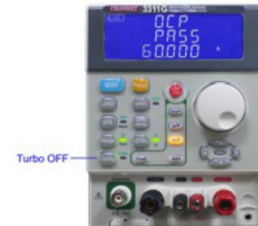
3311G Turbo mode OFF OCP test result screen
