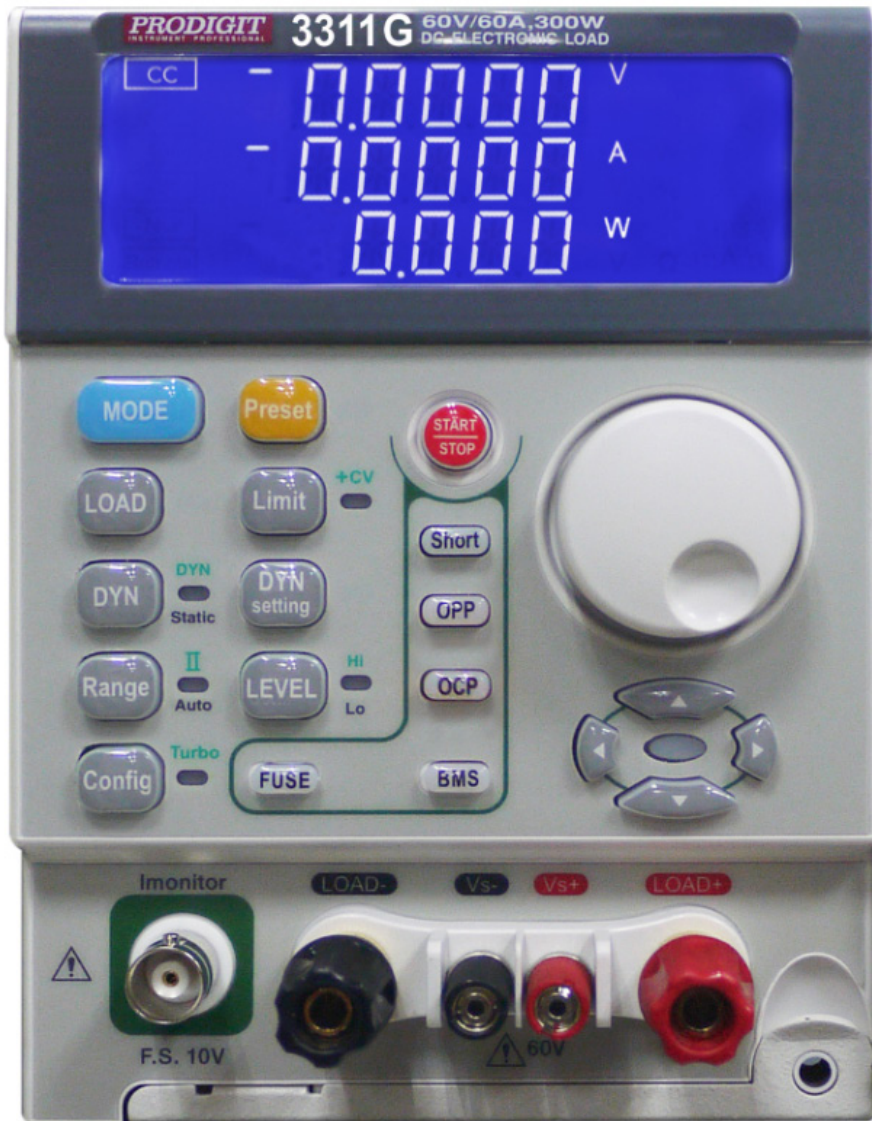
Fig 2-1 Binding post and withdraw handle on the front panel of 3310G series Plug-in load module
