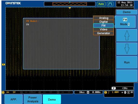
6. Press the *Run* button to display the waveform.
