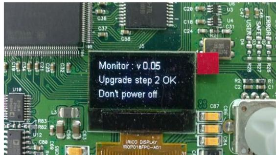
5. Upgrading the firmware is complete. Disconnect the USB cable. Reconnect USB cable and adjust the *Variable* knob to select which model (GDS-3000, GDS-2000A or New GDS Series) the demo board will be used for.
