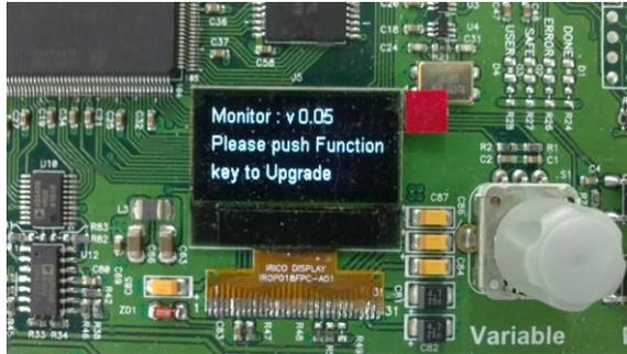
4. Press the *Function* button key to start the procedure. A message on the OLED screen as shown in the photo below will appear during upgrading process.
