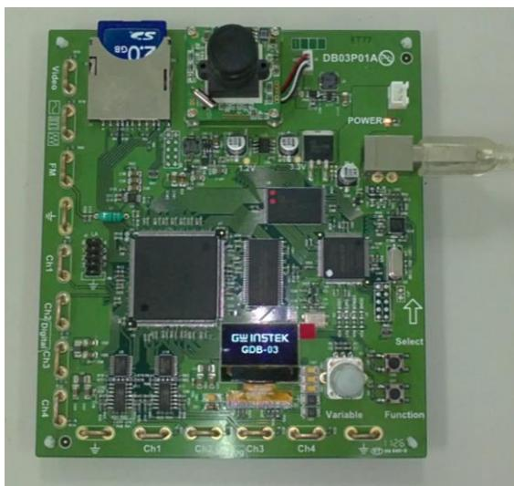
3. When "GW INSTEK" is displayed on the GDB-03 OLED screen, quick turn the *Variable* knob to trigger the firmware upgrading process. A message on the OLED screen as shown in the photo will appear.
