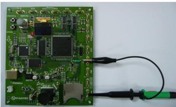
6. Connect the other end of the probe(s) to the corresponding CH1 to CH4 terminals on the GDS-1000B.
