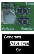
10. Push the *Select* button to change the highlight to the bottom line on the OLED display.
