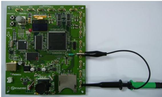
6. Connect the other end of the probe(s) to the corresponding CH1 to CH4 terminals on the GDS-3000.
