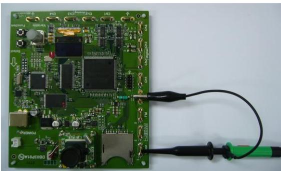
6. Connect the other end of the probe(s) to the corresponding CH1 to CH4 terminals on the GDS-2000A.
