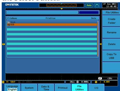
5. Use the Variable knob to select GDB03DemoMode.gz file and then press the Select button to select it.
