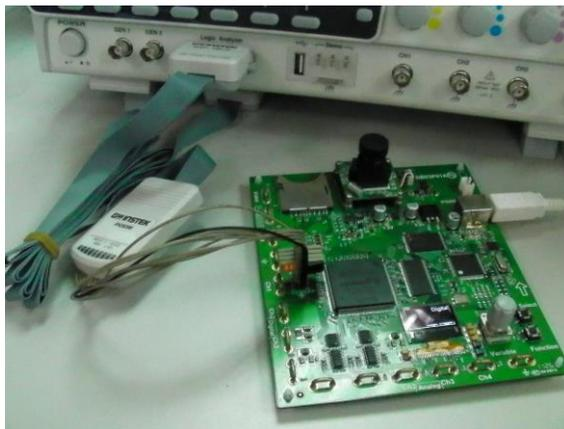
8. Adjust the *Variable* knob on the demo board to select which oscilloscope to demonstrate when the USB cable is connected to the demo board and the oscilloscope. The GDS-2000A is selected when it is highlighted on the OLED display.
