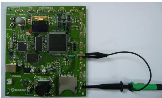
6. Connect the other end of the probe(s) to the corresponding CH1 to CH4 terminals on the GDS-2000E.
