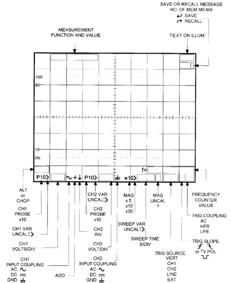
Figure 5-1 Readout Layout
