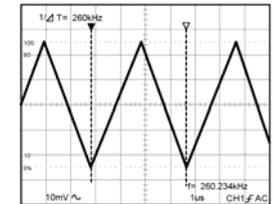
**NOTE.** When the VOLTS/DIV or the TIME/DIV controls are in uncalibrated setting, the  $\Delta V$  and  $\Delta T$  measurement values will be displayed with divisions.
