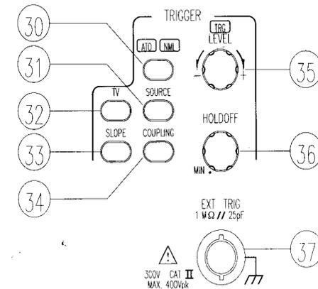
**(30) ATO/NML – Pushbutton and indicator LEDs.**
