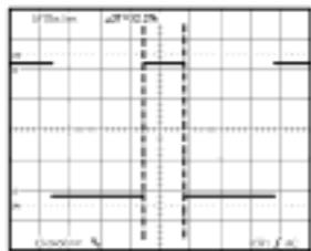
(g).Typical cursor function for phase measurement.
