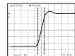
1. Set the VOLTS/DIV and VAR controls to provide an exact five-division vertical display.
