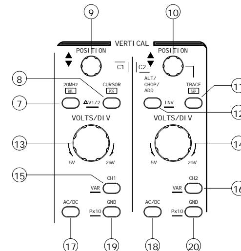
**(7).20MHz BWL** – Pushbutton with indicator LED.
