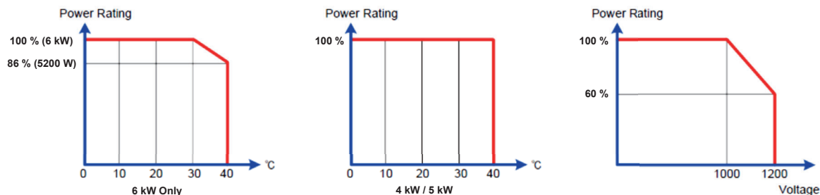
Derating Curve of PEL-5000G 1200 V Model
