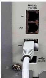
A photograph of the rear panel of a PEL-2000B device. It shows two vertical ports: an RS232/RS485 port with 'IN' and 'OUT' labels above it, and a LAN port below it. A white Ethernet cable is connected to the LAN port. Below the LAN port is a metal ground screw labeled 'GND'. |        |       |       |       |  |
