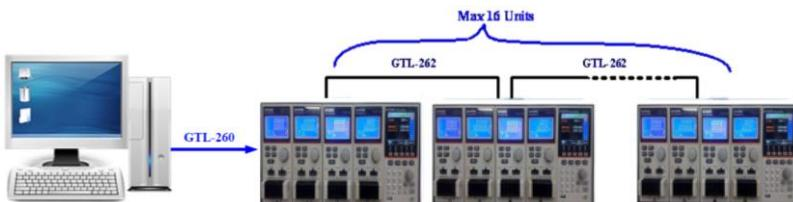
Each unit is assigned a unique address and can then be individually controlled from the host PC.
