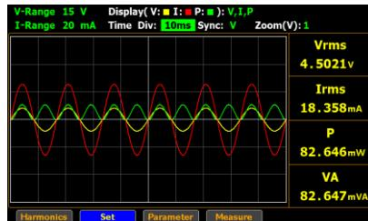
7. Press **Enter** button to enter **Time Div** field. Use up and down arrow keys to toggle between options.
