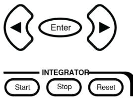
Use the left and right arrow keys to select Integrator mode, and press Enter button to enter the time integrator function. See page 89.
