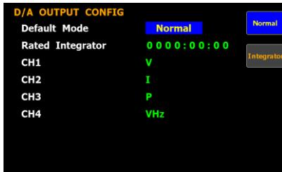
Option      **Normal**      The D/A output parameters for each channel will be changed to the default setting of Normal mode as follows.
