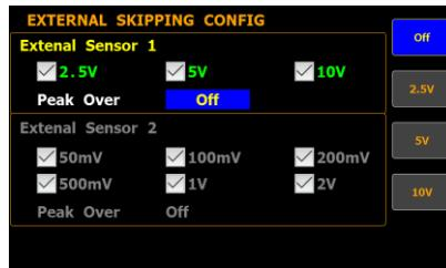
**Option** When the occurrence of peak over-range happens in Auto range mode for external input, user is able to define a measurement range to switch to. The available options for each mode are listed below.
