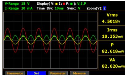
Option           **1, 2, 3** The varied zoom magnifications allow user to customize a preferred waveform graph display. In theory, narrower the measured value, greater the zoom magnification is suitable. In contrast, wider the measured value, smaller the zoom magnification is fitting. The 1 stands for the standard magnification and the 3 represents the highest zoom magnification.
