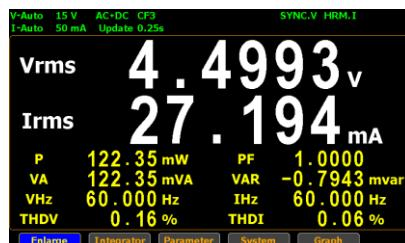
The measured Irms (27.194mA) exceeds the I-Auto 20mA by 130%, so the range is shifted up to 50mA automatically.
