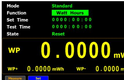
7. Press **Enter** button to enter **Function** field. Use up and down arrow keys to toggle between Ampere Hours and Watt Hours. Press **Enter** button again to confirm your selection.
