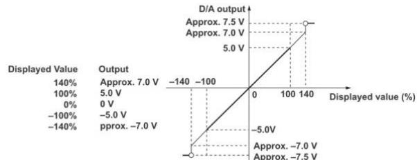
**Examples of D/A Output****Voltage:**
