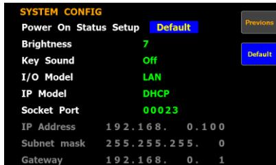
Option **Previous** The status of unit on powering on is set to the status before the last shutdown.
