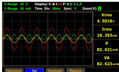
11. Press **Enter** button to enter **Zoom** (V) field. Use up and down arrow keys to toggle between options.
