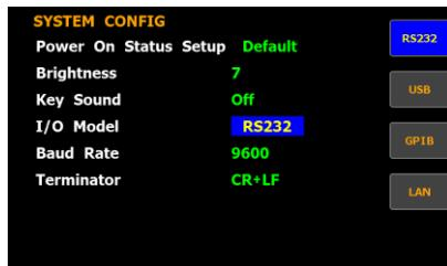
**Option** If interface is set to RS232, the **Baud Rate** and the **Terminator** fields can be selected. For details about configuring RS 232 interface, please see page 136.
