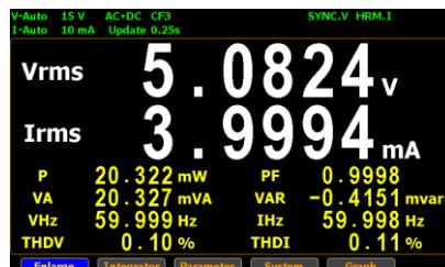
The measured Irms (3.9994mA) is less than 30% of the I-Auto 20mA, so the range is shifted down to 10mA automatically.
