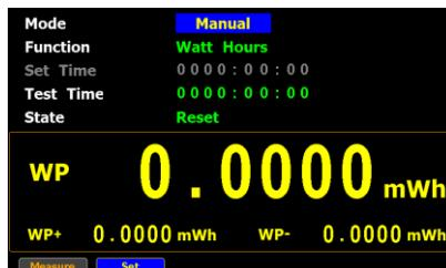
If you select **Standard** or **Continuous** mode, you need to set integrator measurement time before using integrator function. It can be set from 1 second to 9999 hours, 59 minutes and 59 seconds.
