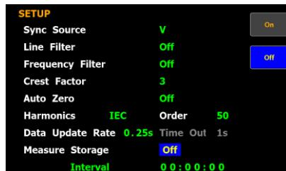
Option      **On**      All measured date will be stored to the internal memory by designated time interval for repeating the storage operation. The **STORE** status icon, for example, on the display lights up in green when Measure Storage function is turn on.
