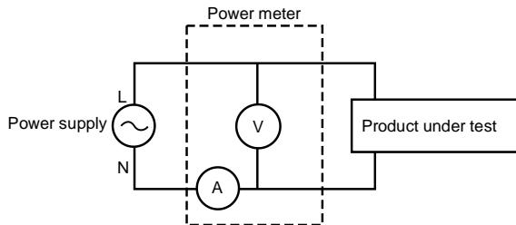
$$\text{Power loss} = (\text{Input voltage[V]})^2 / 2M\Omega$$
