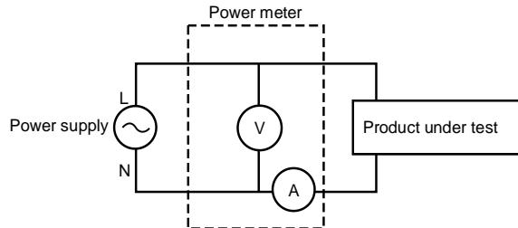
$$\text{Power loss} = (\text{Input current}[A])^2 \times 505\text{m}\Omega$$
