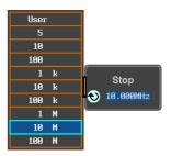
8. Alternatively, select *User* from the list of frequency or press the Select key. Use the arrows to select a base unit and the variable knob to further tune the selected base unit.
