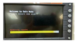
5. When the status indicator shows the complete status (status indicator in yellow completely) and a message of "Update NAND flash success" will appear on the top of status indicator. The firmware upgrading procedure is completed.
