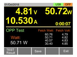
The OPP Test will return the current setting of the last step when the power supply's OPP was tripped.
