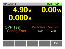
Config Error indicates that the power supply voltage is less than the Trig V voltage setting after the test has started. This can indicate that the power supply output is not on or that the power supply output or Trig V is incorrectly configured.
