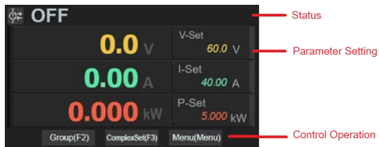
Figure 3-5-1 Source Operating Mode under Standby(OFF)
