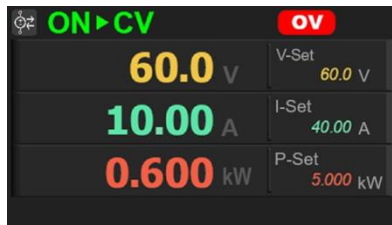
Figure 3-5-2 Source Operating Mode while Output ON, Constant Voltage Mode with Over Voltage alarm triggered
