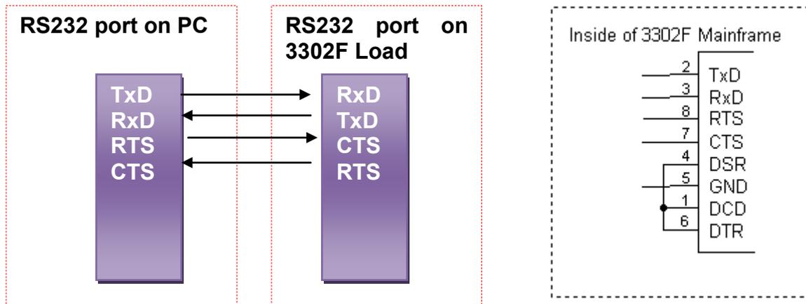
Fig 4-1 RS232 INTERFACE CONNECTION OF REAR PANEL
