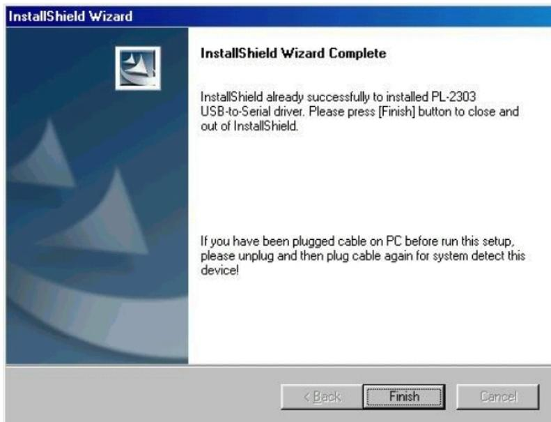
2. After the installation, connect the 3302F and PC with USB. Then select the item USB to Serial Port (COM3), set the BAUD-RATE to 115200bps and the Flow control to Hardware. You should then be able to control the 3302F via USB on COM3.
