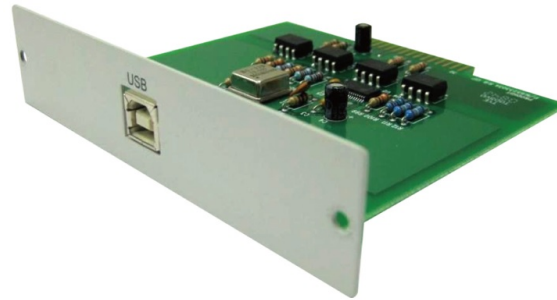
Fig 2-5 36000A Series USB interface
