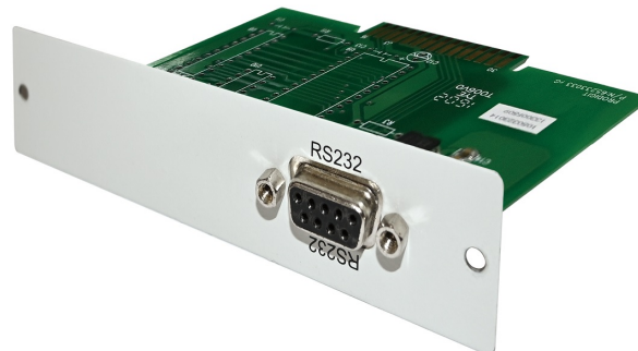
Fig 2-3 36000A Series RS232 interface
