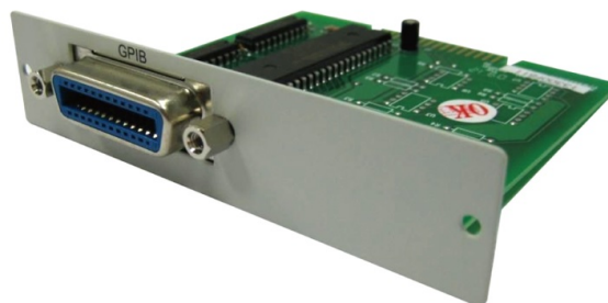
Fig 2-4 36000A Series GPIB interface
