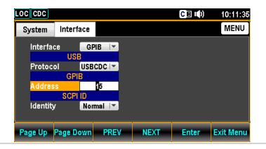
5. Use the Left/Right arrow keys to move the cursor followed by pressing Up/Down arrow keys or press Number keys to define GPIB Address.
