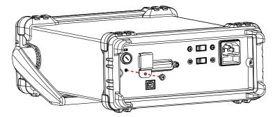
3. Press and hold the fuse holder in the rear panel followed by rotating it counterclockwise with a flat-blade screwdriver.
