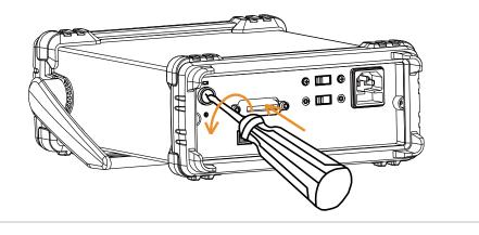
4. The fuse holder comes out. Replace the fuse inserted at the end of the holder followed by rotating the fuser holder clockwise to fasten it firmly.
