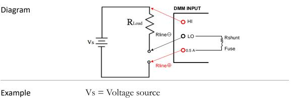
RLoad = Load under test
