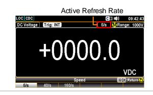
**!** Note The refresh rate cannot be set for capacitance measurement.
