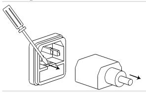
The AC source fuse is stored within the housing.
