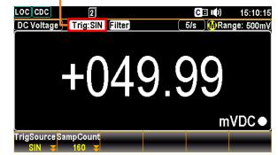
**Change mode** Under SIN (Manual) Trigger mode, press and hold the TRIG button for at least 2 second to return to INT (Auto) Trigger mode.
