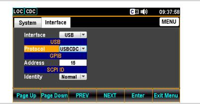
5. Press the F5 (Enter) key or physical Enter key followed by pressing up and down arrow keys to land on the desired USB Protocol option.
