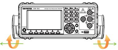
Pull out the handle sideways and rotate it clockwise for the applications below.
