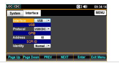
2. Press the F5 (Enter) key or physical Enter key followed by pressing up and down arrow keys to land on the USB option.
