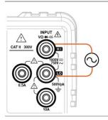
In terms of current, connect test leads between the 0.5 A terminal and the LO terminal or DC/AC 10 A terminal and the LO terminal. The display updates the reading.
