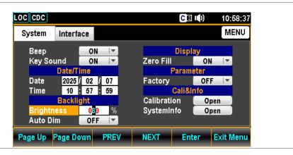
3. Press the F5 (Enter) key or physical Enter key to confirm the input digit for backlight brightness.
