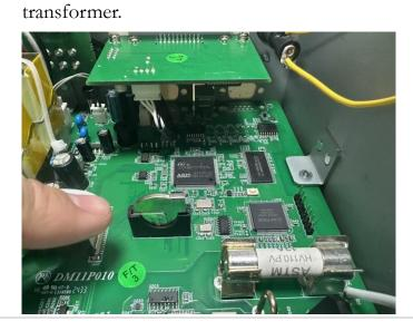
4. Gently remove the metal guard plate on top of the battery followed by pinching the battery out off the compartment with 2 fingers..
