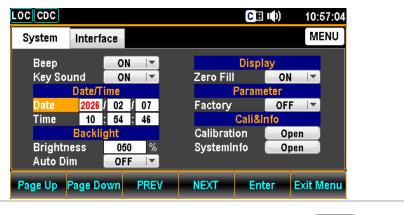
3. Press the F5 (Enter) key or physical Enter key to confirm the input digit for year of Date.
