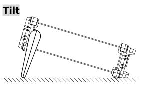
Rotate the handle for tilt stand.
