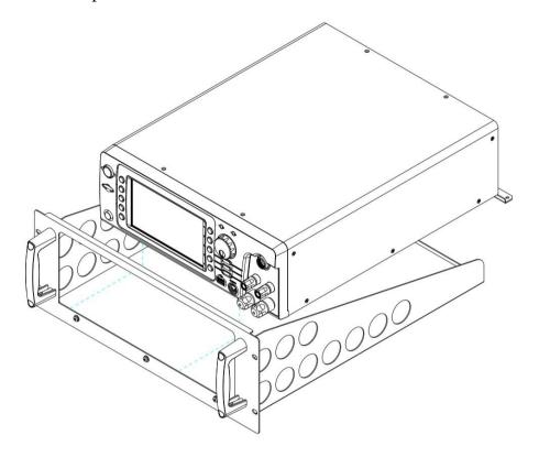
5. Fasten the 2 screws into the L-bracket and the bottom plate firmly to complete assembly.
