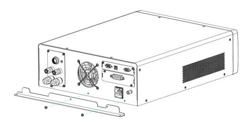
3. Attach the front plate and handles to the bottom plate with fastening the screws.
