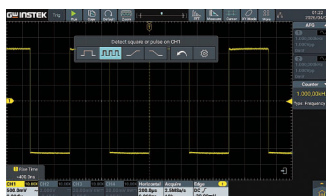
The AUTOSSET Button Automatically Identifies Waveforms
