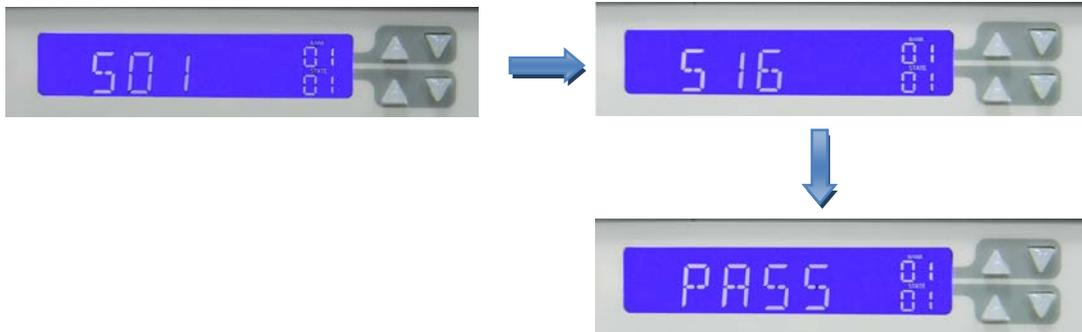
Example 2: Once the edit mode has been used to set the 16 step auto-sequence the user can Press the TEST key. If the test fails at one of the test steps the LCD will flash "NG" And the test will stop. The user can then press ENTER key to continue the test or Press the EXIT button to leave the test mode.
