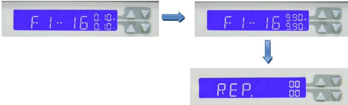
4. The REP function allows the auto-sequence to be repeated a number of times. Both sets of arrow keys are used to set the number of repeats between 0 and 9999 times. Once the Number of repeats has been set press the STORE button to Save the auto-sequence.
