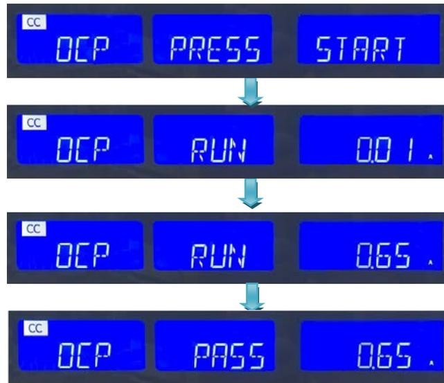
5.10.1.9. The UUT's output voltage drop-out lower than the threshold voltage ( $V_{th}$  Setting), and the OCP trip point is between  $I_{Hi}$  and  $I_{Lo}$  limitation, then Middle 5 digits LCD display will shows "PASS", otherwise shows "FAIL".
