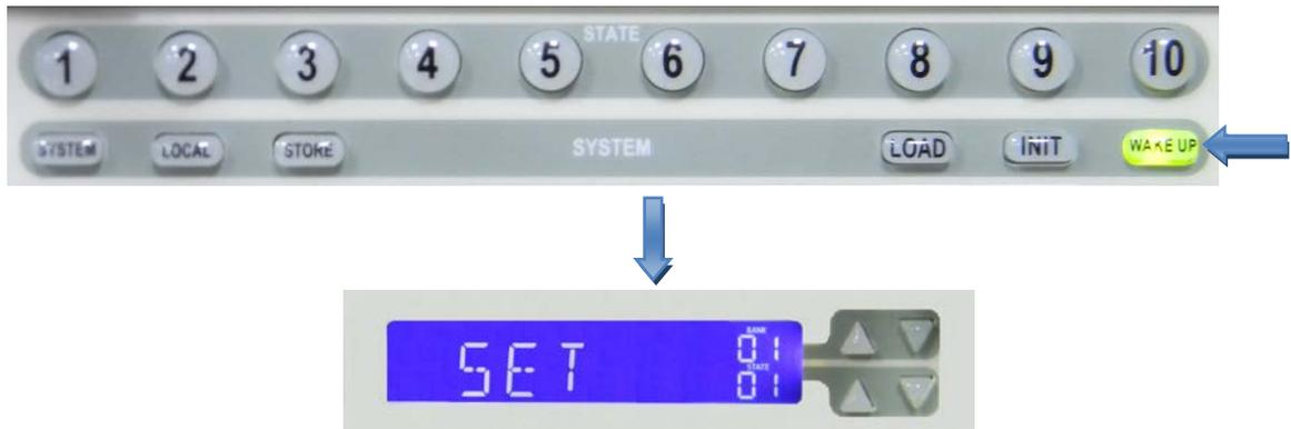
Step 2 Select the memory location (bank and state) that is to be used. Once the Correct location has been selected press the STORE key. This example below Shows bank 01 state 01. After pressing store key the LCD will revert to the Normal message.
