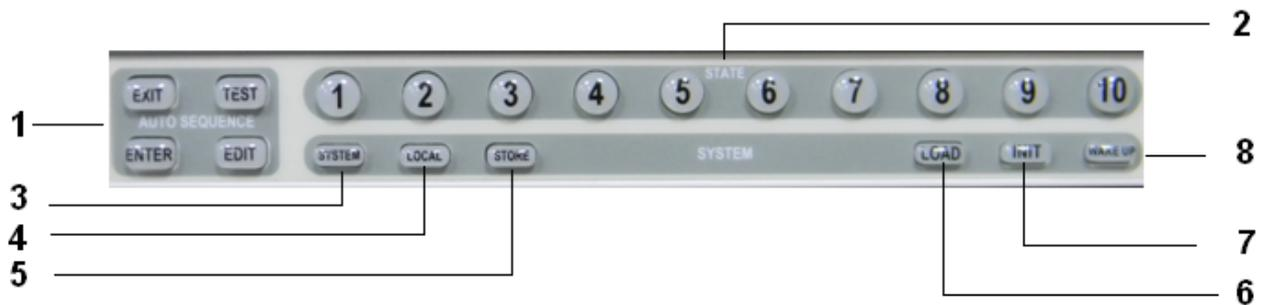
This section briefly describes the buttons on the right hand side of the mainframe. Their Functional use is further described in section 3.4.
