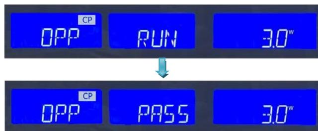
5.11.1.9. The UUT's output voltage drop-out lower than the threshold voltage (V-th Setting), and the OPP trip point is between W\_Hi and W\_Lo limitation, then Right 5 digits LCD display will shows "PASS", otherwise shows "FAIL".
