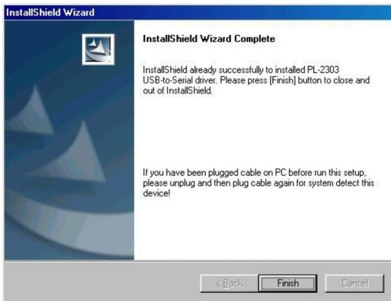
2. After the installation, connect the 3350F and PC with USB . Then select the item USB to Serial Port (COM3), set the BAUD-RATE and Flow control to 115200bps and Hardware to control 3350F with COM3.
