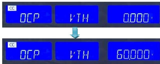
Once the test parameters have been entered the test is started by pressing the red START/STOP button while the OCP PRESS START text is displayed. During the Test The middle LCD will show run and the actual current being Taken will be displayed On the lower LCD
