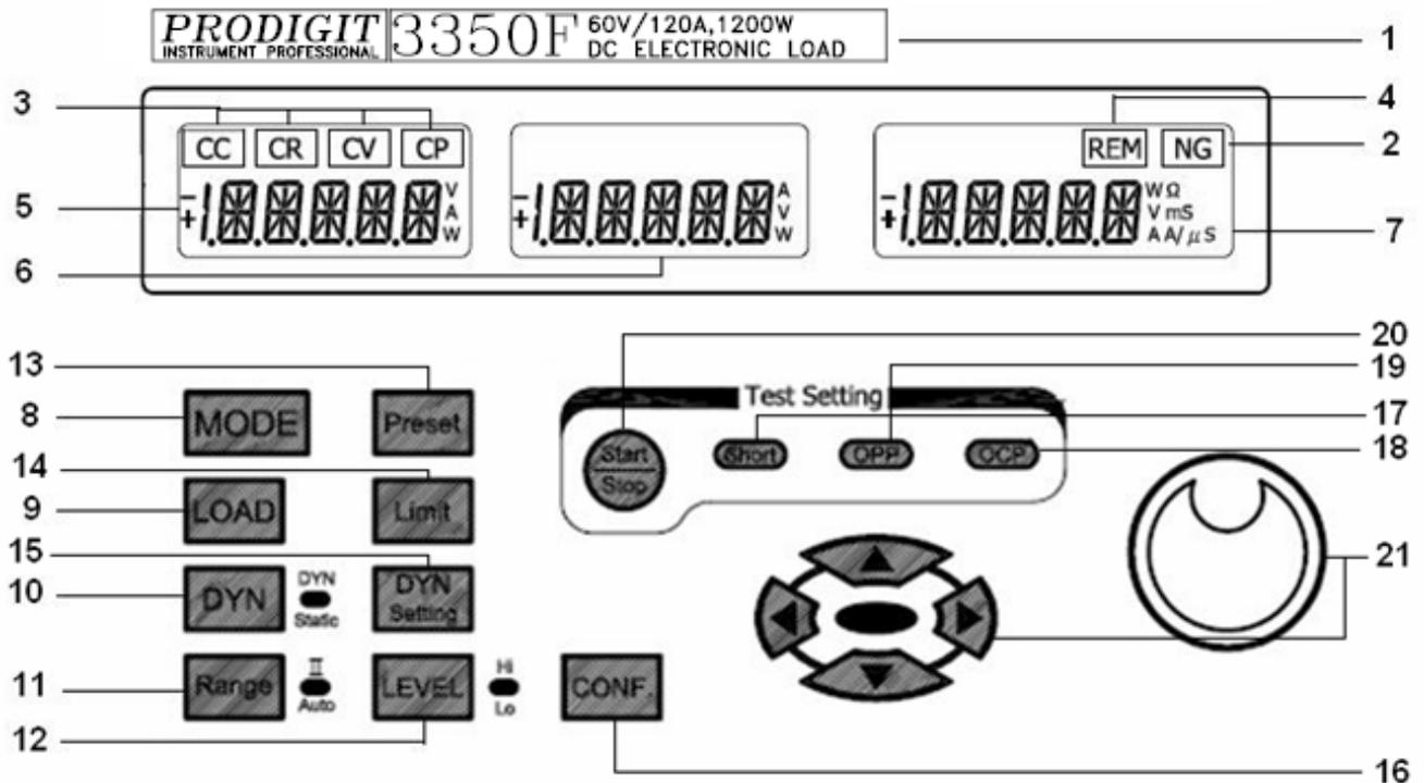
Fig 3-1 3350F-Series High Power Front Panel
