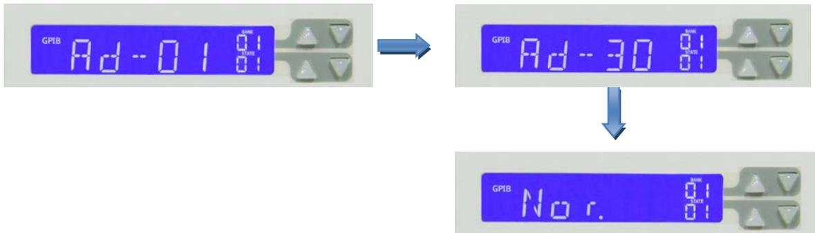
3.5.1.2. To set the RS232 baud rate you must press the system key twice. The LCD will Display the current baud rate. The upper arrow keys are used to change the baud rate. Once the required value is reached press enter or store button to save the new setting. The exit key can be pressed to return to the normal screen.
