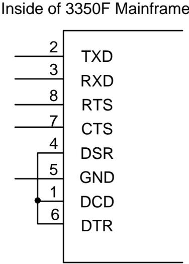
Fig 4-1 RS-232C INTERFACE CONNECTION OF REAR PANEL
