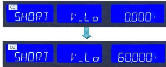
Once the test parameters have been entered the test is started by pressing the red START/STOP button while the SHORT PRESS START text is displayed. During the test the bottom LCD will show run and the actual short Current will be Displayed on the middle LCD.
