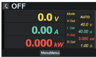
Load Standby State
