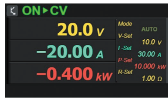
Load Working Mode Operation Interface
