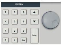
Rotary Knob The ROTARY knob and ARROW keys are used to and ARROW increase or decrease the set values.
