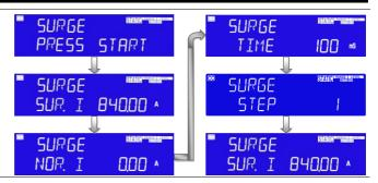
Set SURGE testing surge current, unit is A, setting range 0.00A to full scale.
