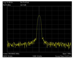
Please note that resolution bandwidth, video bandwidth and frequency span are self-adapted. They adjust to certain values according to frequency span. Sweep time can be self-adapted too.
