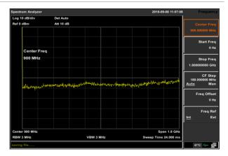
To clearly observe the signal, reduce the frequency span to 1 MHz and set the center frequency to 100MHz.
