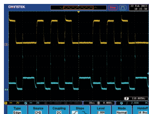
Voltage and Current Waveforms of the Receiving Signals of a Cellular Phone
