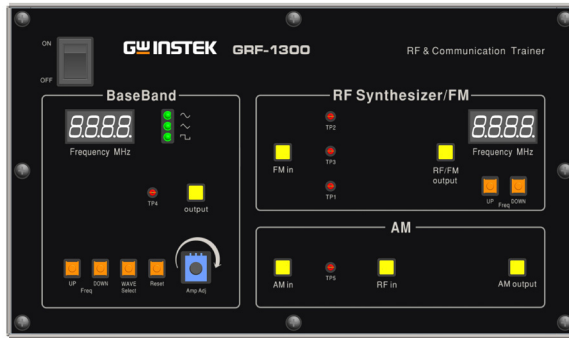
Figure A-1. The GRF-1300 control panel
