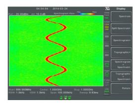
The Spectrogram view shows signals in both the frequency and time domain. The X-axis represents frequency, the Y-axis represents time and the color of each point represents the amplitude at a particular frequency & time (Red = high  $\rightarrow$  dark blue = low).
