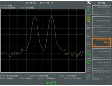
The example below shows the same signal with the gated sweep timed to sweep when only the desired frequency is output.
