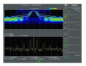
Displays both topographic and spectrum views of the signal.
