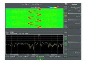
Displays both spectrographic and spectrum views of the signal.
