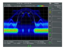
The topographic view shows the frequency of events. The topographic view is useful for observing smaller signals that have been overpowered by stronger signals or to easily observe intermittent events. Color is used to represent the frequency of an event. Red represents a high frequency of occurrence, while blue represents events that occur rarely.
