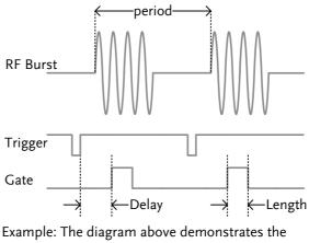
relationship between the input trigger, the input signal and the position of the gated sweep relative to the input signal.
