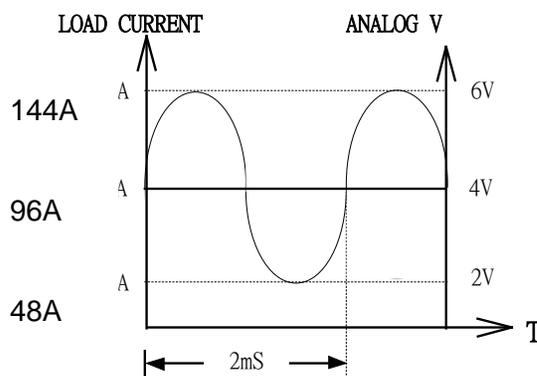
Fig 2-8 Analog programming load current in CC mode operation
