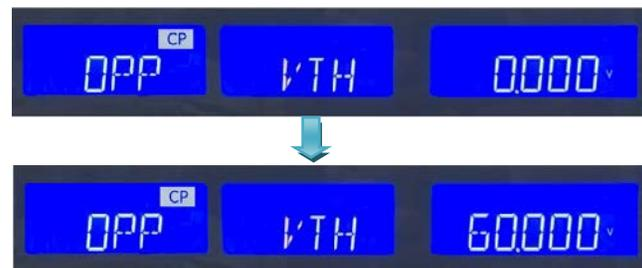
Once the test parameters have been entered the test is started by pressing the red START/STOP button while the OPP PRESS START text is displayed. During the Test the middle LCD will show run and the actual power being taken will be Displayed on the lower LCD.
