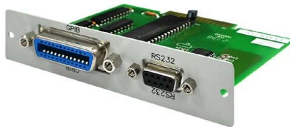
Fig 2-7 33501F GPIB & RS232 Connection
