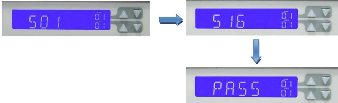
Example 2: Once the edit mode has been used to set the 16 step auto-sequence the user can press the TEST key. If the test fails at one of the test steps the LCD will flash "NG" and the test will stop. The user can then press the ENTER key to continue the test or press the EXIT button to leave the test mode.
