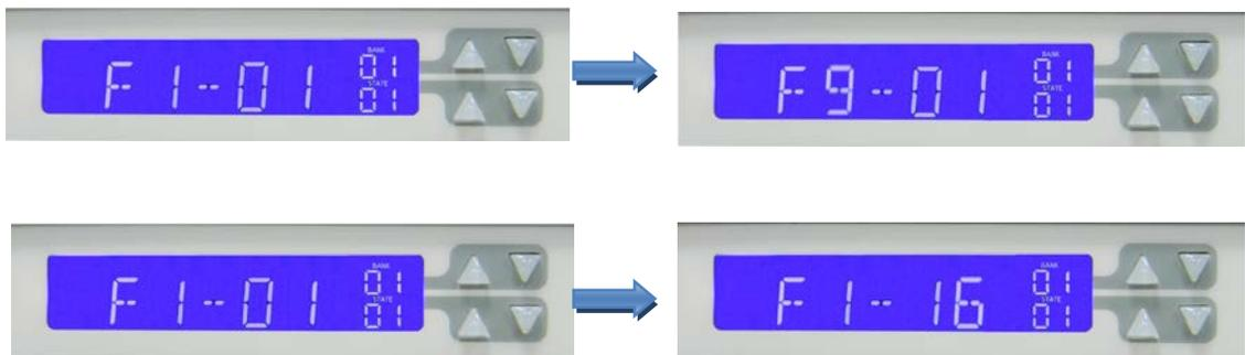
2. Once the auto-sequence number has been selected the Memory location of the First test step can be selected. The Arrow keys next to the 3350F LCD are used to Select the Memory BANK and Memory STATE.
