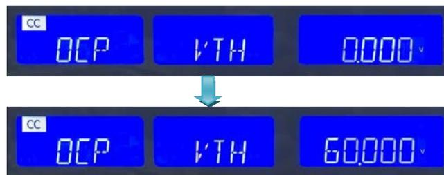
Once the test parameters have been entered the test is started by pressing the red START/STOP button while the OCP PRESS START text is displayed. During the Test The middle LCD will show run and the actual current being Taken will be displayed On the lower LCD
