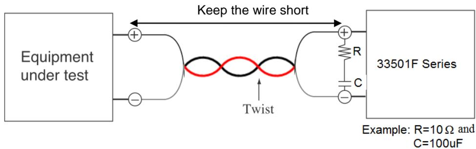
Fig 2-13 Length of wiring
