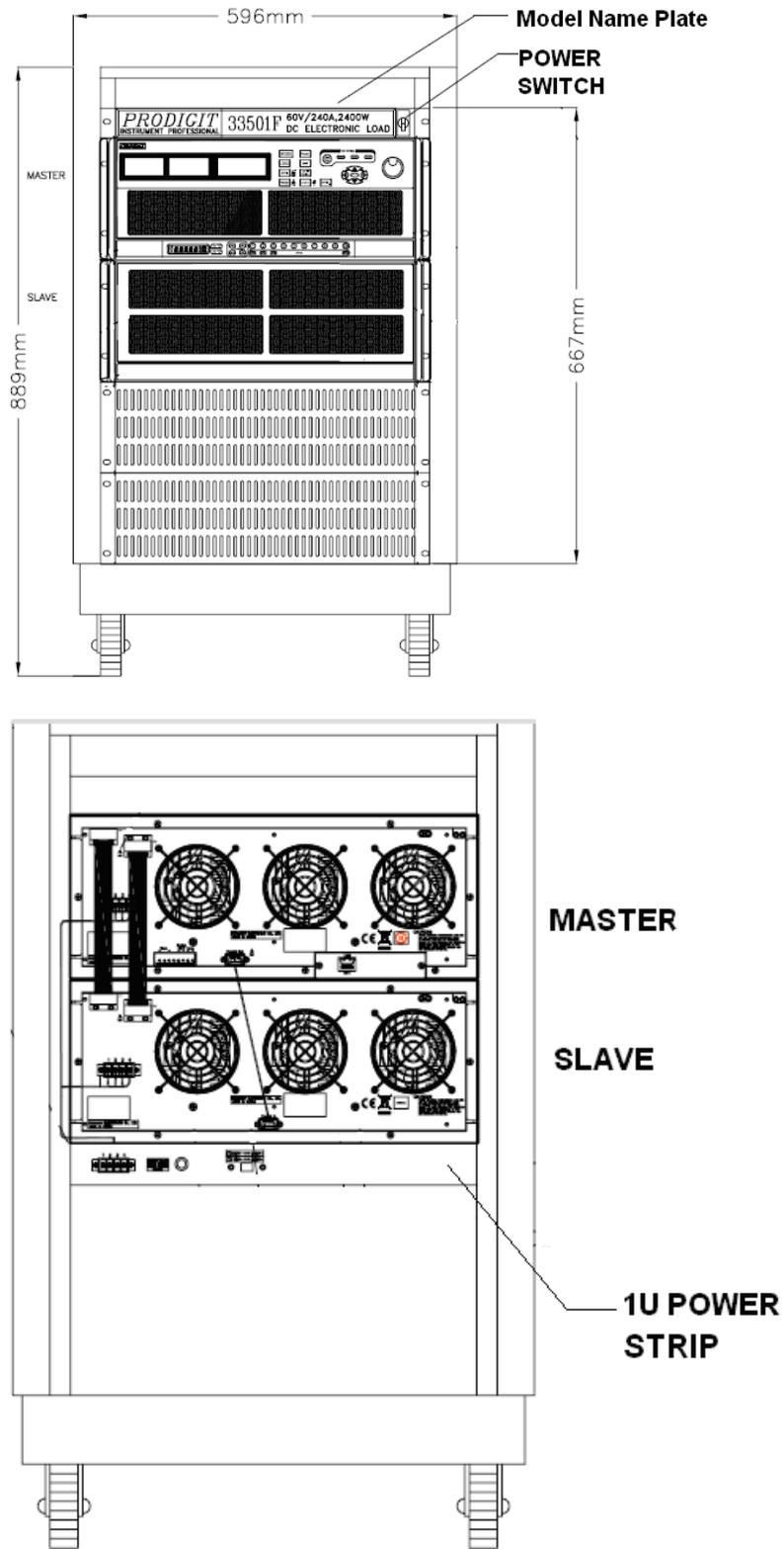
Fig 3-2 33501F Series High Power electronic load
