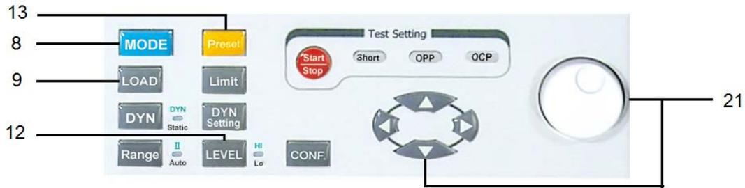
Example: PSU 5 V / 3 A, CC mode, Level HI 3.000A, Level 1.500A
