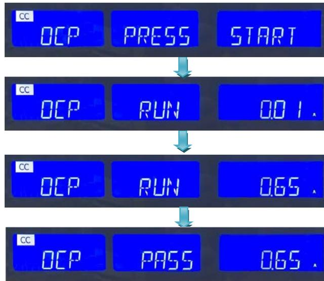
5.10.1.4. The UUT's output voltage drop-out lower than the threshold voltage (V-th Setting), and the OCP trip point is between I\_Hi and I\_Lo limitation, then Middle 5 digits LCD display will shows "PASS", otherwise shows "FAIL".
