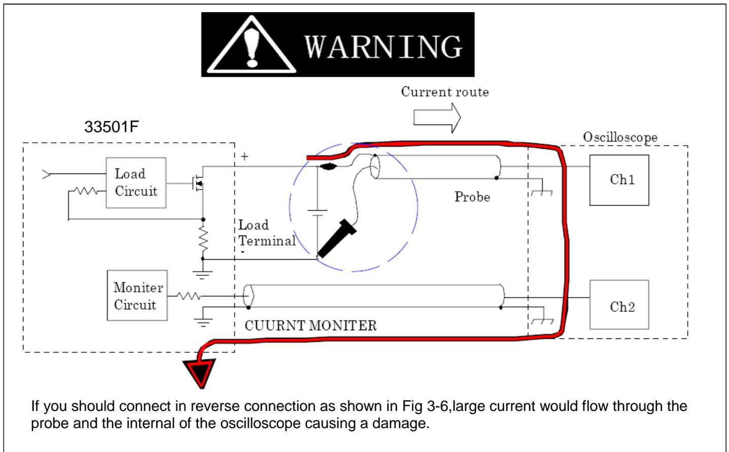
Fig 3-6 (Wrong) Connections to an oscilloscope
