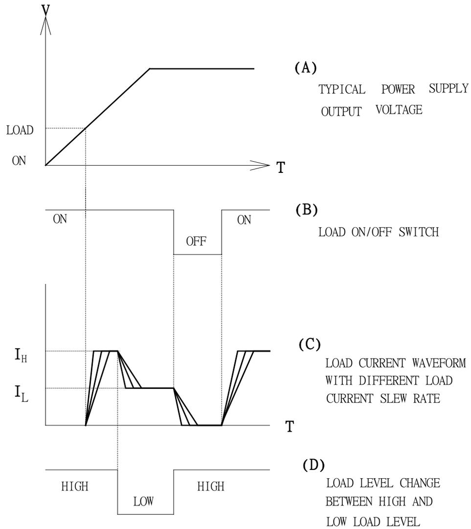
Fig 2-9 The relationship of load current load ON/OFF, load level and output voltage of DC power Supply at turn ON
