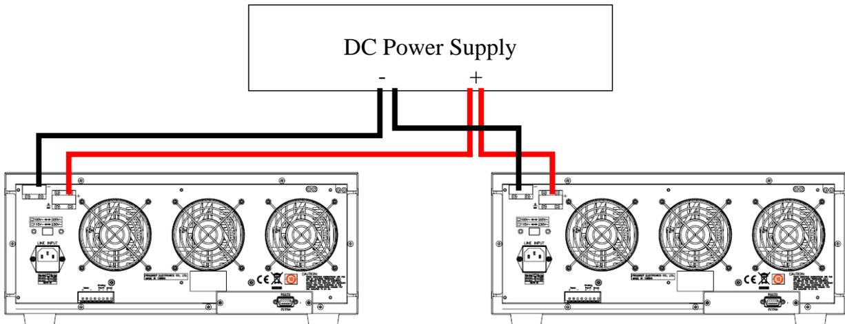
Fig 5-10 Parallel operation connection
