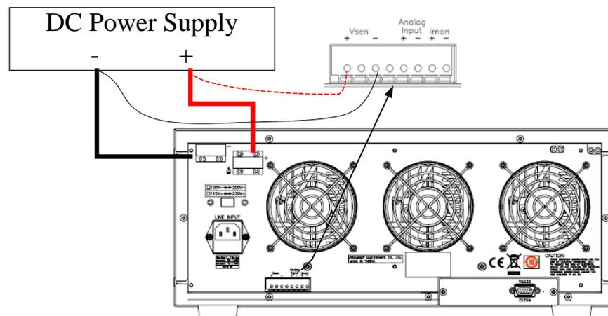
Fig 3-3 Remote sense connection on front panel
