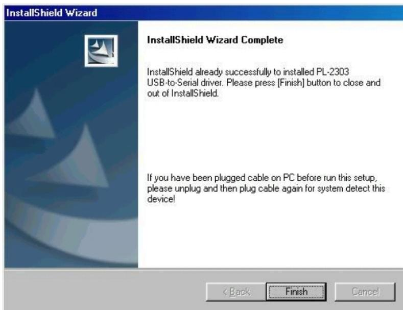
2. After the installation , connect the 33501F Series and PC with USB . Then select the item USB to Serial Port (COM3) , set the BAUD-RATE and Flow control to 115200bps and Hardware to control 33501F Series with COM3.
