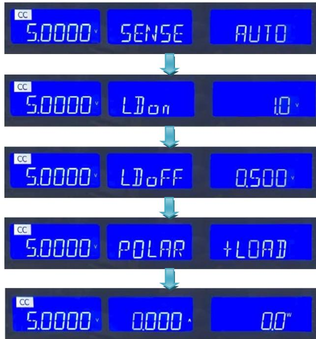
Note 1: The adjustable LDon (LOAD ON) voltage is valid for CC, CR & CP operating Modes. The adjusted LDon voltage will not operate in CV mode.
