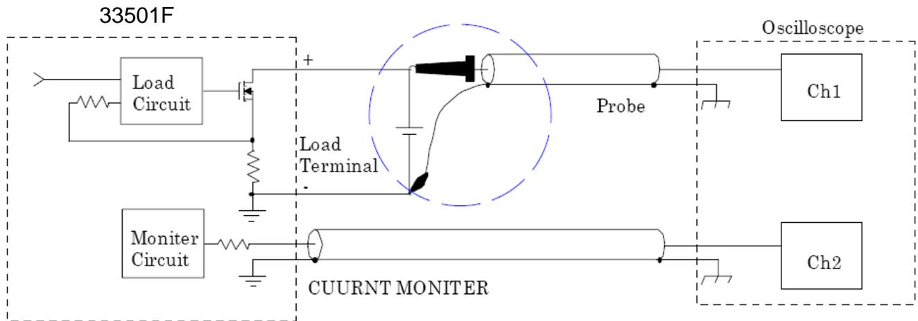
Fig 3-5 (Correct) Connections to an oscilloscope
