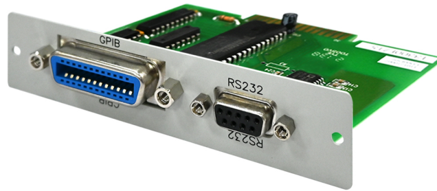
Fig 2-7 3360F GPIB & RS232 Connection
