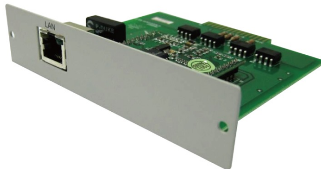
Fig 2-6 3360F LAN Connection Rear panel
