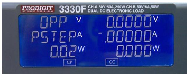
4.12.5.4. Press up key, set stop load watt 3.25W, press OPP key to the next step.
