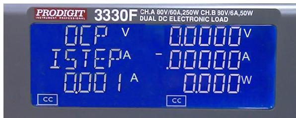
4.11.5.4. Setting stop load current 0.65A, press OPP key to the next step.
