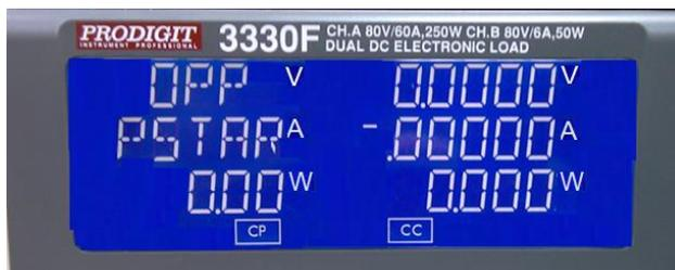
4.12.5.3. Press up key, set step load watt 0.02W, press OPP key to the next step.
