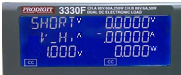
4.13.5.4. Press down key, setting V-Lo voltage to 0V, press Short key to the next Step.
