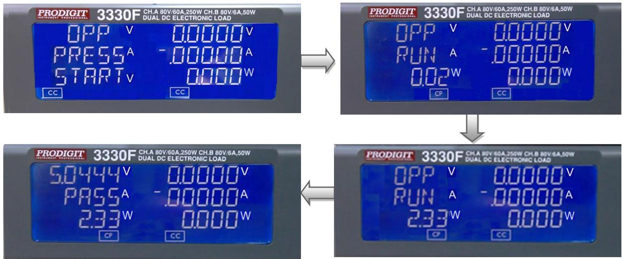
4.12.5.7. the UUT's output voltage drop-out lower than the threshold voltage (V-th setting), and the OPP trip point is between W\_Hi and W\_Lo limitation, then lower 5 digits LCD display will shows "PASS", otherwise shows "FAIL".
