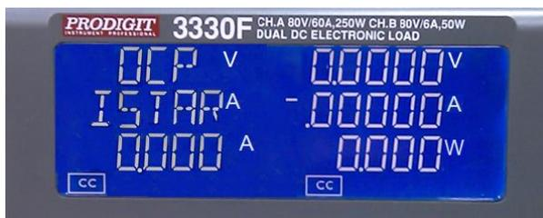
4.11.5.3. Setting step load current 0.001A, press OPP key to the next step.
