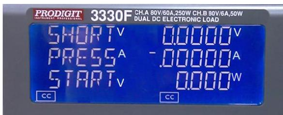
4.13.5.2. Press UP key, setting Short time to 10000ms, press Short key to the next Step.
