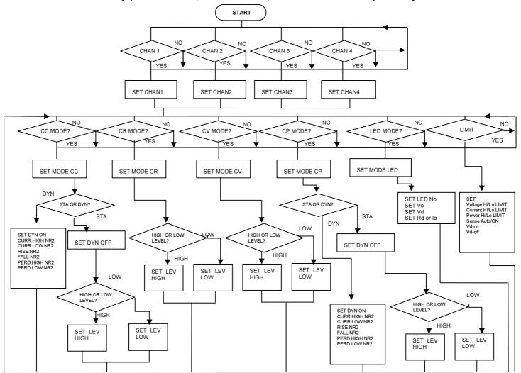
Fig 2-3 3342G series electronic load module load condition setting flow chart
