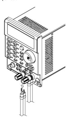
Fig 3-8 Hook Terminal Y type large size terminal connections
