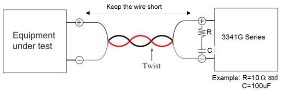
Fig 2-5 Length of wiring
