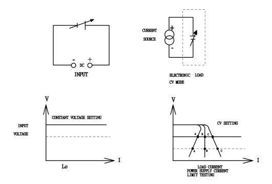
Fig 4-5 Constant Voltage mode application
