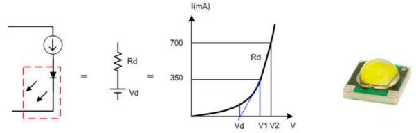
Fig 4-8 LED's equivalent circuit and characteristic curve
