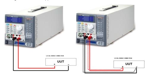
Fig 3-2 typical connection of 3342G series load module
