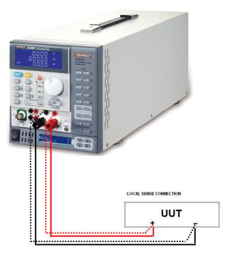
Fig 4-2 Remote voltage sense connections
