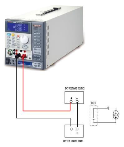
Fig 4-15 Zero-Volt loading connection
