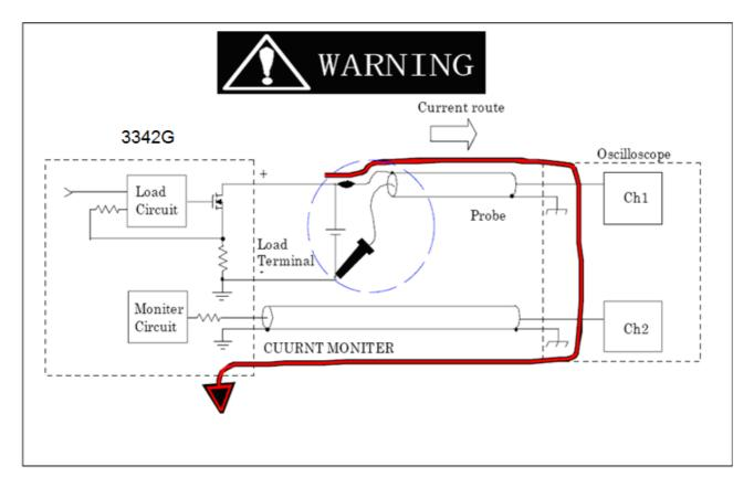
If you should connect in reverse connection as shown in Fig 3-6, large current would flow through the Probe and the internal of the oscilloscope causing a damage.
