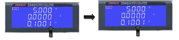
Knob Right key: Setting digit can flash Knob Right key to push down setting value move Right one-digit.
