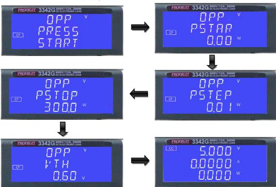
PSTAR: setting the start power, The LCD display shows 「OPP」 on upper 5 digit LCD display, Middle 5 digit LCD display 「PSTAR」, lower 5 digit LCD display setting value, the unit is "W", the setting range is 0.00W to the full scale of the CP mode specification. The setting is by rotating the setting
