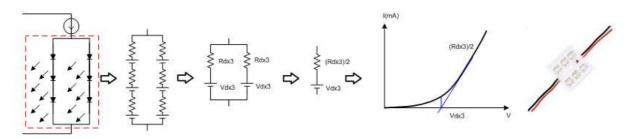
Fig 4-11 Several LED cascading and parallel connection and characteristic curve
