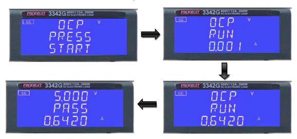
4.12.1.8. the UUT's output voltage drop-out lower than the threshold voltage(V-th setting), and the OCP trip point is between I\_Hi and I\_Lo limitation, then middle 5 digits LCD display will shows "PASS", otherwise shows "ERROR".
