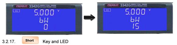
The SHORT key allows the parameters of a SHORT circuit test to be entered. The SHORT test will attempt to sink high current up to the 3342G load module's maximum current in order to check the power source's protection and behavior. The test time can be adjusted and threshold values for the High and low voltage limits set.
