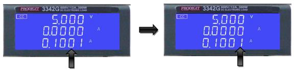
Knob up key: Setting digit can flash Knob UP KEY to push down add setting value.
