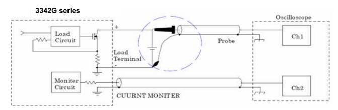
Fig 3-5 (Correct) Connections to an oscilloscope
