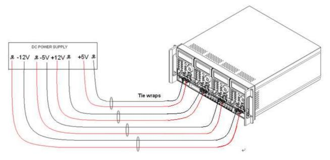
Fig 4-13 Connection between 3342G series plug-in load and multiple output power supply
