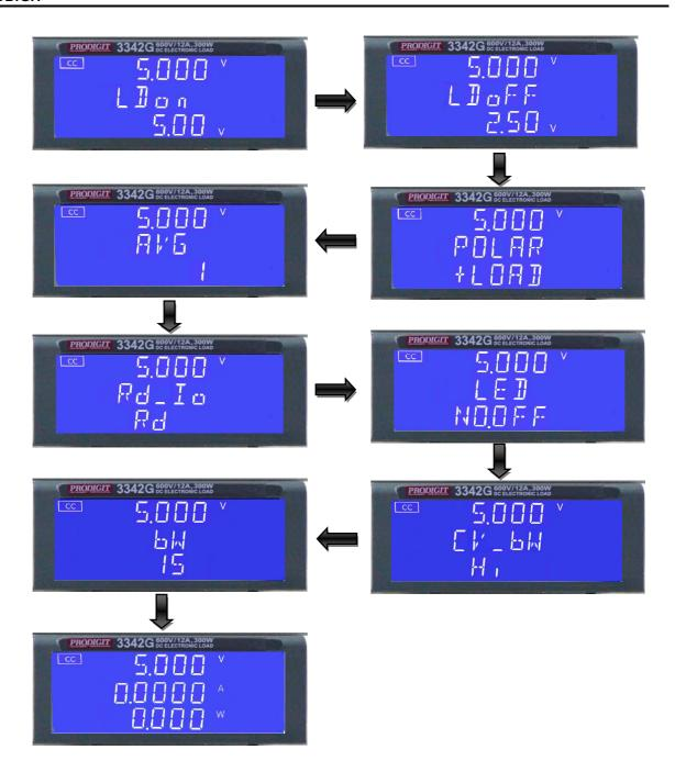
Set Load ON voltage, the middle of the 5 digit LCD display will show "LDon", Lower 5 digit LCD display will show setting value, the units is V, The Load ON Voltage set range from 0.00V to 50.00V step 0.01V by rotating the setting knob. If the load is greater than the input voltage Load ON voltage setting, the Electronic load current begin to load on.
