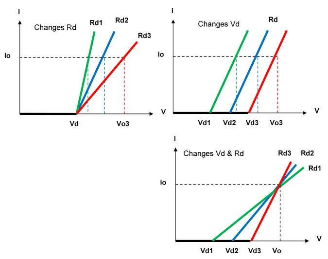
Fig 4-12 LED MODE operation mode of the application
