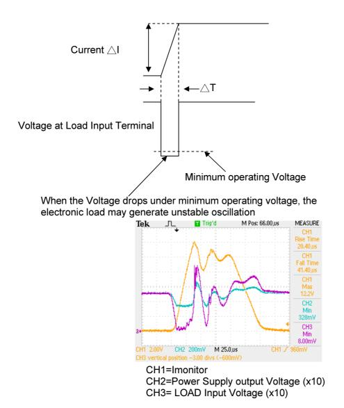
Fig 2-4 Waveform example: Generate unstable oscillation
