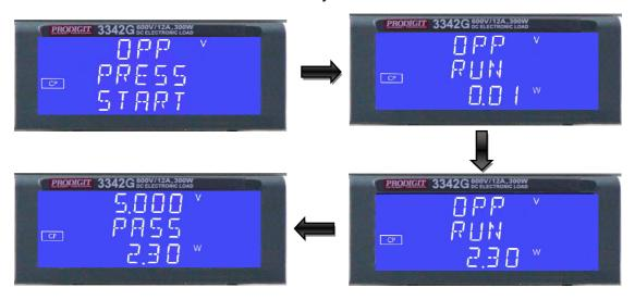
4.13.1.8. the UUT's output voltage drop-out lower than the threshold voltage (V-th setting), and the OPP trip point is between W\_Hi and W\_Lo limitation, then lower 5 digits LCD display will shows "PASS", otherwise shows "FAIL".
