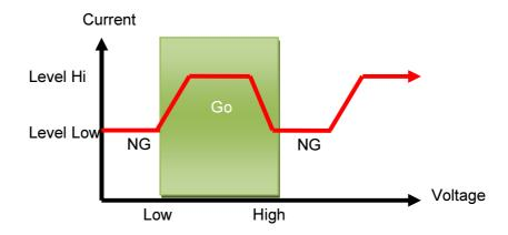
CR mode, press limits key to set the V-Hi and V-Lo voltage upper and lower limits of the GO / NG.
