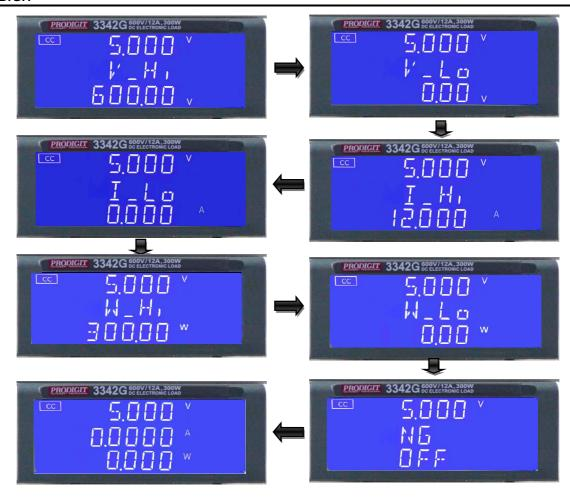
Setting Upper limit voltage VH, Middle 5 digit LCD display 「V-Hi」,lower 5 digit LCD display the unit is "V", The V-Hi set range from 0.00 V to 300.00V step 0.01V by rotating the Setting knob.
