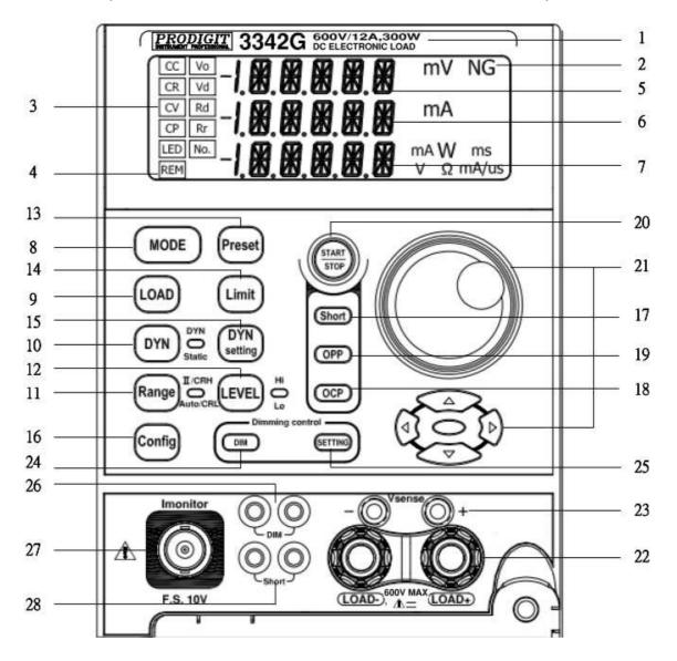
Fig 3-1 Front panel of 3342G plug-in module
