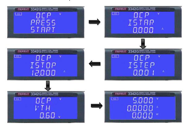
• ISTAR: setting the start current point, The LCD display shows 「OCP」 on upper 5 digit LCD display, Middle 5 digit LCD display 「ISTAR」,lower 5 digit LCD display setting value, the unit is "A".
