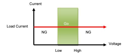
CC Dynamic Mode, press key to set the Level Hi and Level Low voltage upper and lower limits of the GO / NG.
