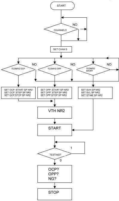
Fig 4-16 3342G series electronic load OCP, OPP, SHORT operation flow chart
