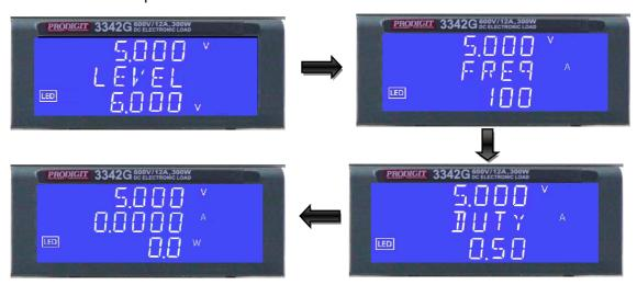
LEVEL setting, The LCD display shows, lower 5 digit LCD display, the unit is "V", the setting range is 0.000V to the 12.000V of the LED mode specification, Step 0.04V by rotating the setting knob.
