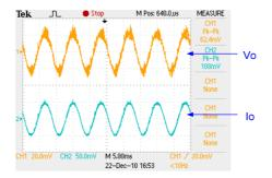
Fig 4-9 LED Driver ripple
