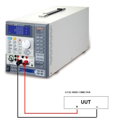
Fig 4-1 Local voltage sense connections
