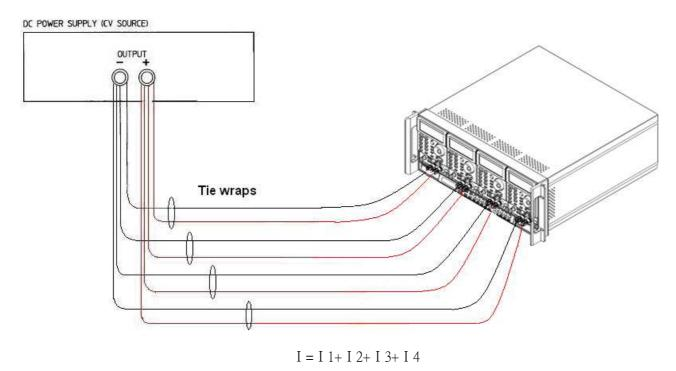
Fig 4-14 3342G series plug-in module parallel operation
