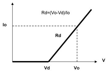
Fig 1-8 LED mode characteristics
