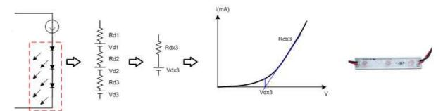
Fig 4-10 3 LED cascading connection equivalent circuit and characteristic curve
