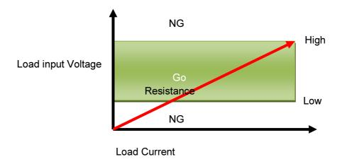
CV mode, press limits key to set the I-Hi and I-Lo Current upper and lower limits of the GO / NG.
