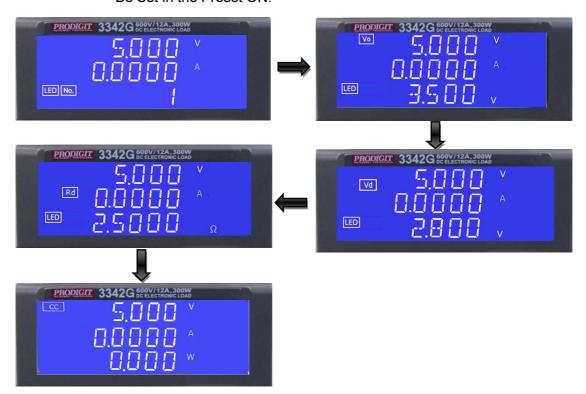
LED Mode, LED Quantity set the initial value of 1, Simulation can change this setting LED cascading connection features a few pieces, the latter setting the specifications of LED can be set a parameter, cascading connection LED as a light Bar, to set back the settings, 3342G~ 3343G setting range is 1~90,
