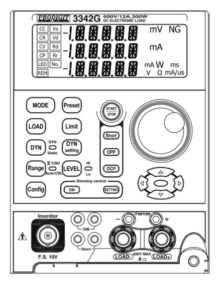
Fig 2-1 Binding post and withdraw handle on the front panel of 3342G series Plug-in load module
