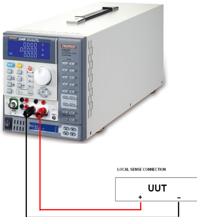
Fig 4-1 Local voltage sense connections
