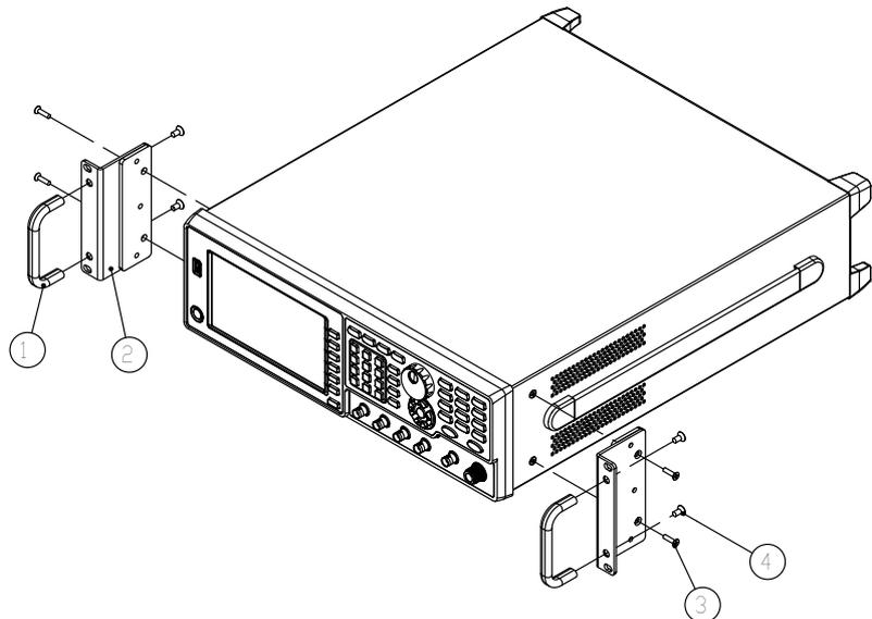
4. The GRA-447 rack mount is assembled with the GSG-2000 unit completely.
