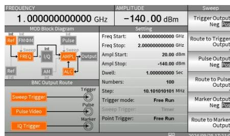
As shown in the diagram below, When the F5 key is pressed, the BNC output route will display on the left lower corner of the Sweep setting page.
