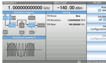
2. To change the FM modulation waveform, press the F3 key and a key next to the waveform it indicates. When a waveform is selected, the waveform name will be highlighted in bold font. For example, when the Sine waveform is selected, the waveform **Sine** will become bold.
