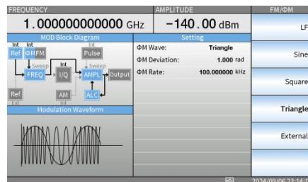
2. Press the F1 soft key to set the  $\Phi M$  Deviation and press the F2 soft key to set the  $\Phi M$  Rate.
