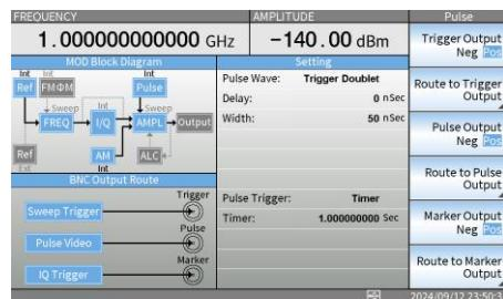
As shown in the diagram below, When the F6 key is pressed, the BNC output route will display on the left lower corner of the Pulse setting page.
