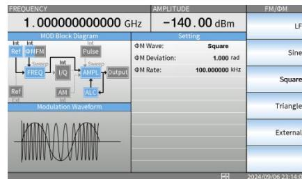
2. Press the F1 soft key to set the ΦM Deviation and press the F2 soft key to set the ΦM Rate.
