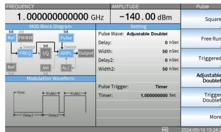
2. Press the F1 soft key, the F2 soft key, the F3 soft key, and the F4 soft key to set the Delay, Width, Delay 2, and Width 2 of the adjustable doublet waveform, respectively.
