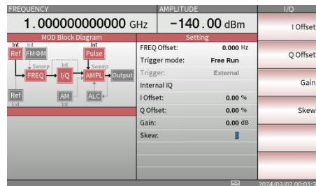
**External IQ input** 10. To select internal IQ input, press the F2 key. Then you will see the further option about external IQ modulation input appears as shown in the figure below.
