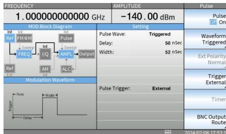
6. Press the F1 key to activate Pulse modulation. Press the F1 key again to disable Pulse modulation. When Pulse modulation is activated, the Pulse key will light on, and you will see the Pulse icon in the MOD Block Diagram turning blue, as shown in the figure below.
