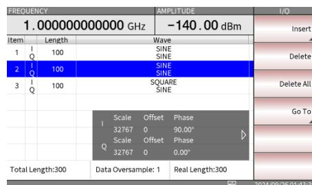
4. Use the scroll knob and arrow keys to select the waveforms for both channels I and channel Q and edit their corresponding parameter (including Scale, Offset, Phase, Duty, Symmetry), and edit Length for waveforms. Press the F6 key to apply it.
