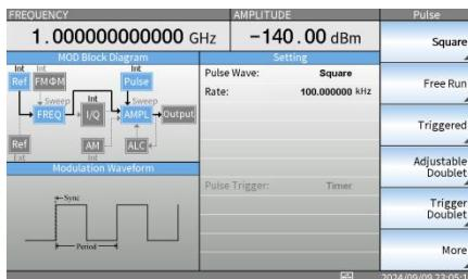
2. Press the F1 soft key to set the Rate of square waveform.
