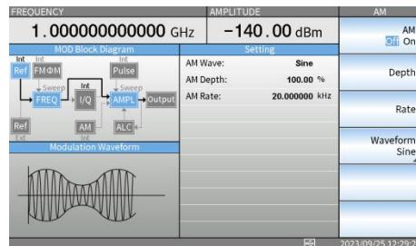
2. Press the F1 key to activate the AM modulation. Press the F1 key again to disable it. When AM modulation is activated, the AM key will light on, and you will see the AM icon in the MOD Block Diagram turning blue, as shown in the figure below.
