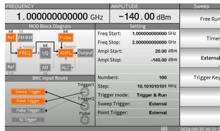
6. Press the F1 key to select polarity. There are polarities positive and negative. You can see the difference from the BNC input route diagram.
