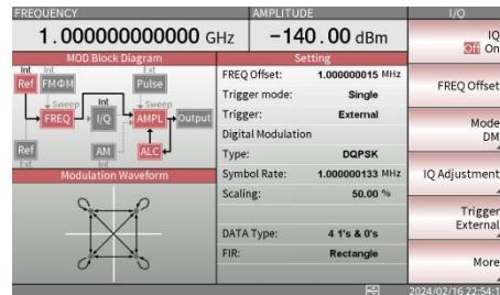
2. Press the F1 key to activate the Vector modulation. Press the F1 key again to disable the Vector modulation. When the Vector modulation is activated, the I/Q key will light on, and you will see the I/Q icon in the MOD Block Diagram turning brown, as shown in the figure below.
