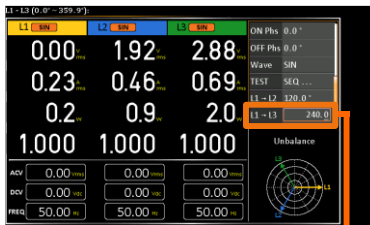
L1 -> L3 Phase degree setting
