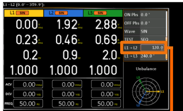
L1 -> L2 Phase degree setting
