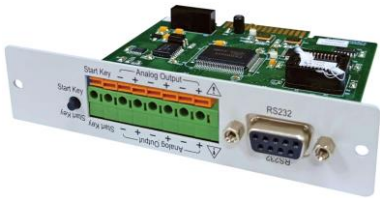
PEL-5000G series 9923 Current Waveform Generator & RS232 Interface
