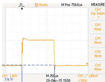
Figure F PEL-5006G-150-600 BMS overcharge flow test program diagram (single pulse)
