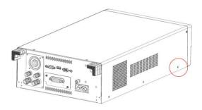
3. Attach the 4 L-type brackets using the 594B-W3008NS1 screws to the unit.
