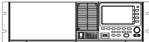
GRA-439-E Rack Mount Diagram (ASR-2000R)
