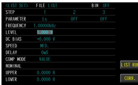
3. Use the numeric keypad to enter the test voltage/current.
