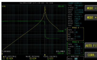
3. Use option key on the right of the LCD screen to select the appropriate equivalent circuit model.
