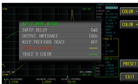
3. Use option key on the right of the LCD screen to select a desired color.
