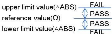
$\Delta\%$  The difference between the measured value and the NOMINAL value is compared with the percentage of the NOMINAL value.
