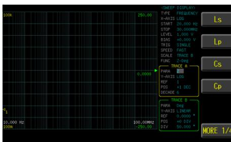
3. Use option key on the right of the LCD screen to select a parameter for this sweep item.
