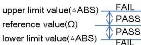
$\Delta\%$  The difference between the measured value and the NOMINAL value is compared with the percentage of the NOMINAL value.
