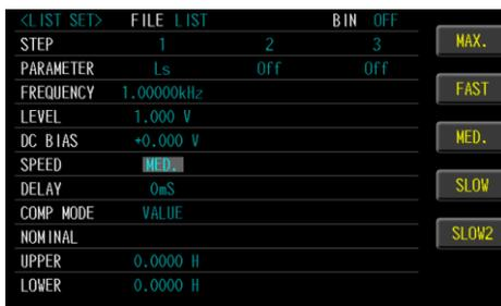
3. Use option key on the right of the LCD screen to select a test speed item.
