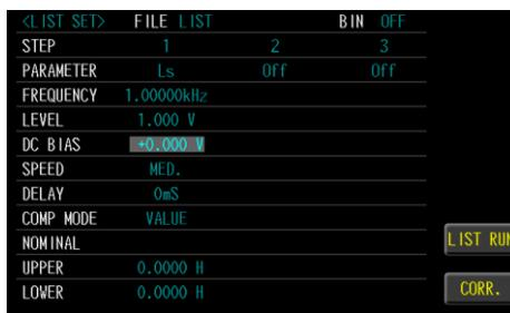
3. Use the numeric keypad to enter the test DC Bias.
