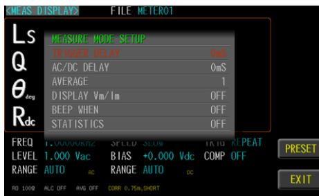
3. Use key pad to input delay timer value ,unit is ms.
