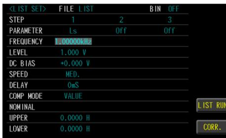
3. Use the numeric keypad to enter the test frequency.
