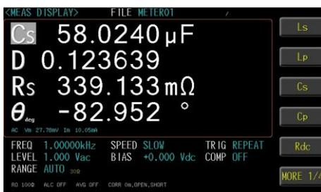
3. Use option key on the right of the LCD screen to select a parameter for this measurement item.
