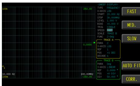
3. Use option key on the right of the LCD screen to select a speed mode for this sweep item.
