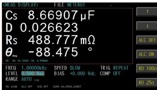
3. Use option key on the right of the LCD screen to adjust the level value or use the numeric keypad to enter the test level and select ALC/RO for this measurement item.
