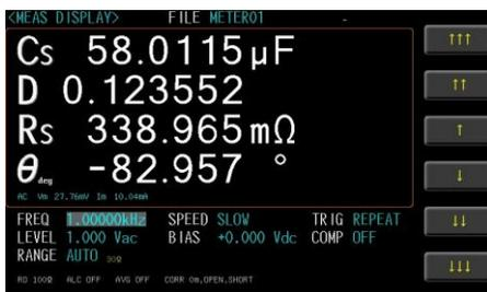
3. Select option key on the right of the LCD screen to adjust the frequency value by rough or minor adjusting method or use the numeric keypad to enter the test frequency.
