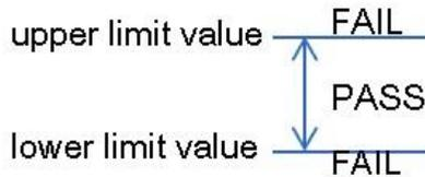
△ The difference between the measured value and the NOMINAL value is compared.
