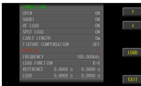
3. Use option key on the right of the LCD screen to select ↑or↓ item switch point number.
