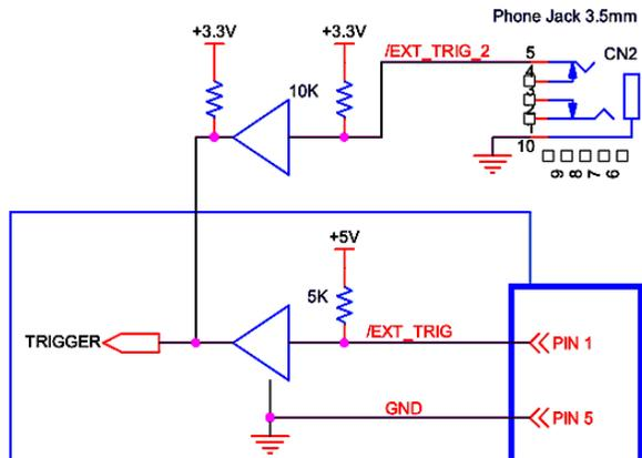
Connection method for input circuit
