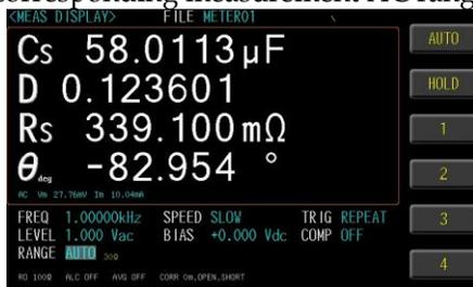
3. Use option key on the right of the LCD screen to select a desired measurement range.
