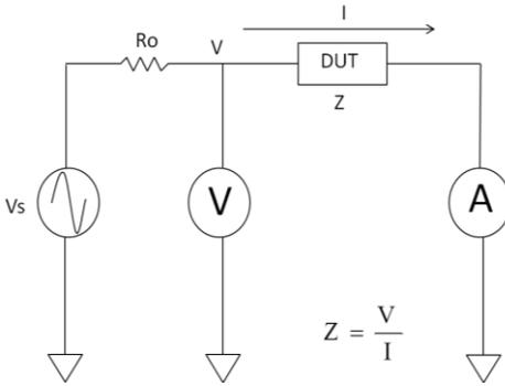
The simplified model of the LCR-8200 series impedance measurement,  $V_s$  is the test signal voltage and  $R_O$  is source resistance. If the current across the DUT is  $I$  when a test signal voltage  $V$  is applied, the DUT's impedance,  $Z$ , is expressed by  $Z = \frac{V}{I}$ . Impedance,  $Z$ , contains real and imaginary parts. The figure shows vector representation of impedance as follow.
