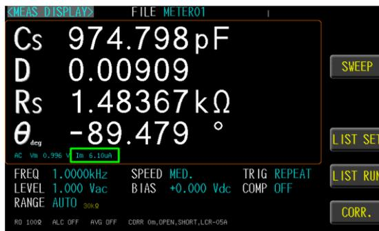
Available range is from 0.01 to 20000 with the unit of uA. This item is only available when TRIGGER MODE is set in AUTO mode.
