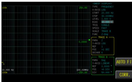
3. Use the numeric keypad to enter the test DC BIAS or Vac/Iac and unit.
