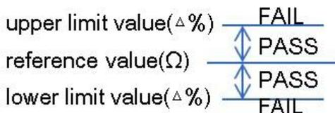
12. The LIST test BIN sort results below the LCD screen.
