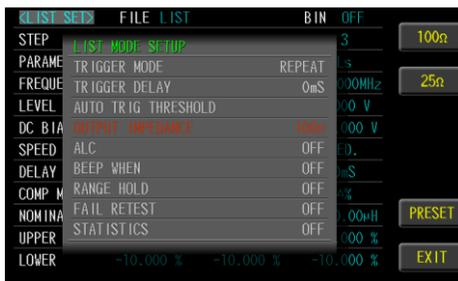
3. Use option key on the right of the LCD screen to select an impedance item.
