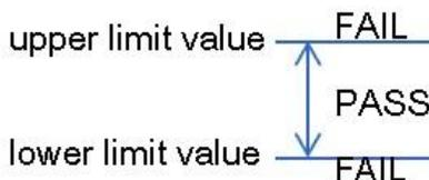
$\Delta$  The difference between the measured value and the NOMINAL value is compared.
