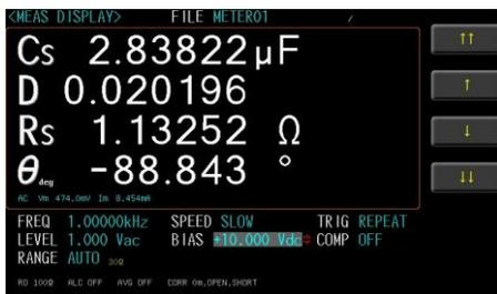
3. Select option key on the right of the LCD screen to adjust the frequency value by rough or minor adjusting method or use the numeric keypad to enter the DC Bias voltage.
