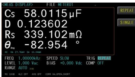
3. Use option key on the right of the LCD screen to select a trigger mode for this measurement item.
