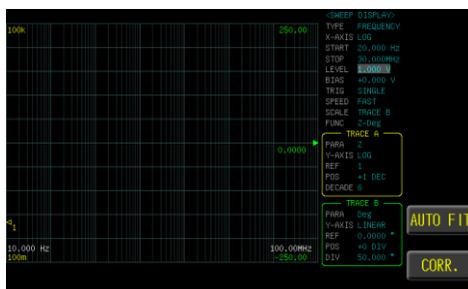
3. Use the numeric keypad to enter the test Vac/Iac (frequency) or Freq. (Vac/Iac/DC BIAS) and unit.
