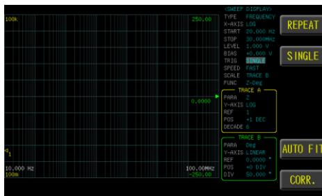
3. Use option key on the right of the LCD screen to select a trigger mode for this sweep item.
