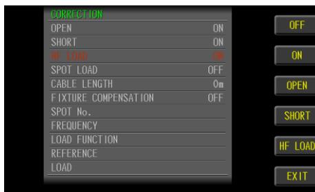
3. Use option key on the right of the LCD screen to select **HF LOAD** item to start execution.
