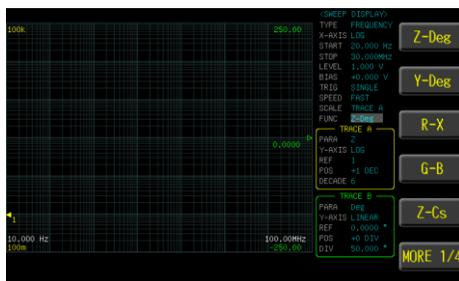
3. Use option key on the right of the LCD screen to select a function type for this sweep item.
