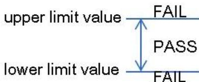
**Δ** The difference between the measured value and the NOMINAL value is compared.
