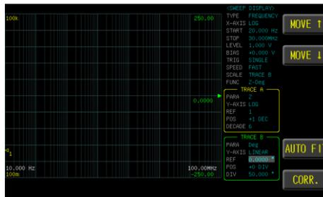
3. Use option key on the right of the LCD screen to select a scale type for this sweep item.
