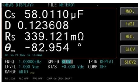
3. Use option key on the right of the LCD screen to select a test speed for this measurement item.
