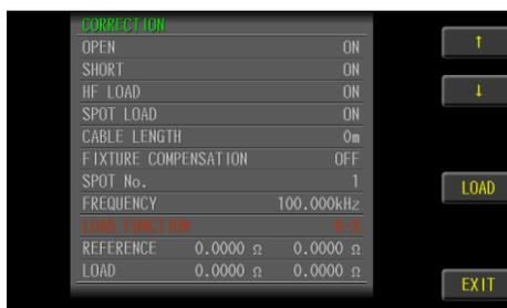
3. Use option key on the right of the LCD screen to select ↑ or ↓ item switch function.
