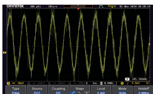
Unfiltered Waveform with Noise Interference
