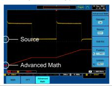
Position and Unit To move the math waveform vertically, press *Position* and use the Variable knob.
