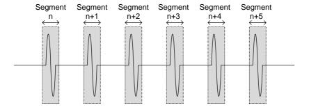
As shown below, the memory is divided into segments to increase the number of events that can be effectively captured with the same acquisition memory. Also notice that the scope doesn't need to rearm the trigger between each segment, this makes the segmented memory function especially useful for high speed signals. The time between each segment is also recorded so that accurate signal timing can also be measured.
