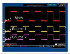
Position and Unit To move the math waveform vertically, press the *Position* key from the side menu and use the Variable knob to set the position.
