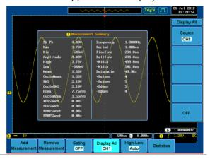
Remove Measurements To remove the measurement results, press *OFF*.
