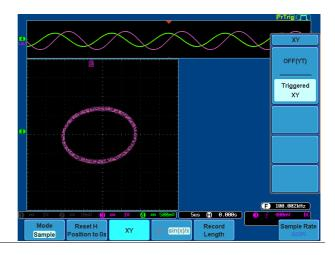
To move the X Y waveform position, use the vertical position knob: Channel 1 knob moves the X Y waveform horizontally, Channel 2 knob moves the X Y waveform vertically. Similarly, the X2 and Y2 axis can be positioned using the channel 3 and channel 4 vertical position knobs.
