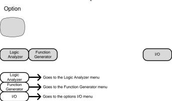
\*Note: Any option that is not installed will be grayed-out.
