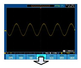
1. Press the relevant function key again to reduce the bottom menu. For example: press the Trigger Menu key to reduce the trigger menu.
