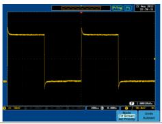
8. Select Vector Waveform Press the *Display* key, and set the display to *Vector* on the bottom menu.
