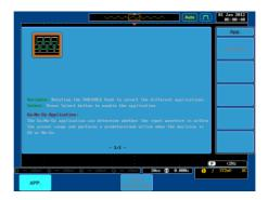
4. When the desired application is highlighted, press *Uninstall* to begin the uninstallation. Press again to confirm.
