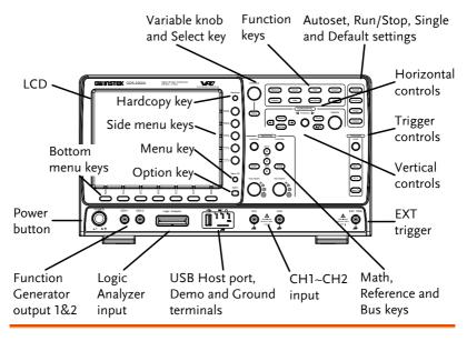
LCD Display 8" SVGA TFT color LCD. 800 x 600 resolution, wide angle view display.
