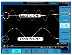
In the example above, the file label for channel 1 is displayed next to the channel indicator and is also displayed in the *Save Waveform* menu. The Ref\_1 file label is shown next to the reference indicator.
