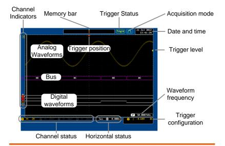
Analog Shows the analog input signal waveforms.
