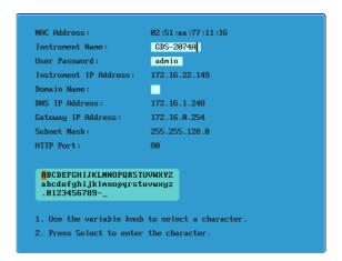
6. Use the *Up* and *Down* arrows on the side menu to navigate to each Ethernet configuration item.
