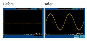
3. To undo Autoset, press *Undo Autoset* from the bottom menu.
