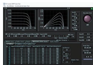
PV Inverter Mppt Auto Test
