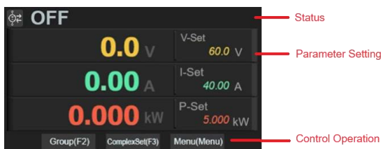
Figure 3-5-1 Source Operating Mode under Standby(OFF)
