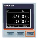
In order to prevent the DUT from being damaged by any person other than the user changing the setting parameters at will, the user can activate the panel lock function to protect the safety of the DUT.
