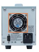
The product uses a temperature-controlled fan, whose speed will change with the temperature inside the machine, so that the temperature inside the machine remains stable and the specifications will also be stable.
