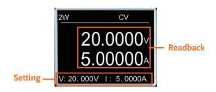
The set value and the actual readback value after the output is turned on can be displayed directly on the screen at the same time.
