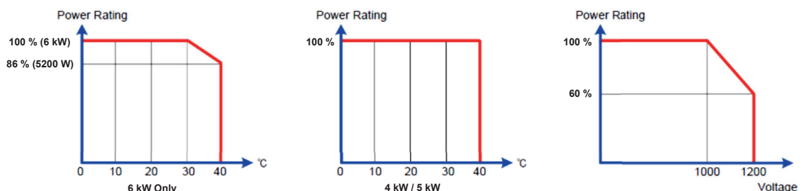
Derating Curve of PEL-5000G 1200 V Model
