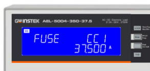
Turbo : OFF, Fuse mode Test result screen
