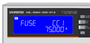
Turbo ON, Fuse mode Test result screen
