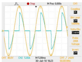
90 degree SCR Leading edge current waveform
