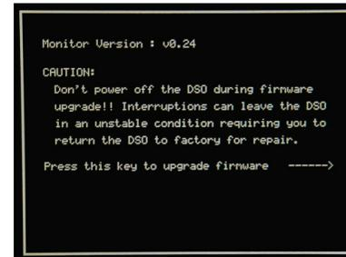
3. Upgrading the firmware. Press the F4 key. The oscilloscope automatically starts upgrading the firmware. When the status indicator at the bottom of the display shows the "Upgrade Success!!" message, upgrading the firmware is completed.
