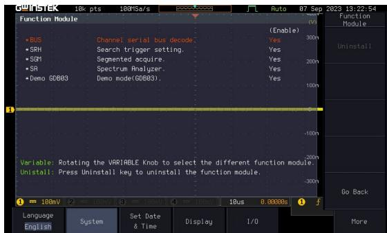
Professional version of MPO-2000B's installed function module
