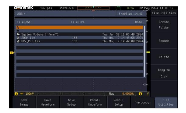
4. Find and select the upgrade license file to install. Press the "Select" key (front panel) to install the license.
