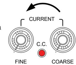
3. Turn the current coarse and fine knobs to the centered position
