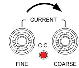
7. Turn the current coarse and fine knobs to the centered position
