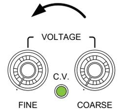
5. Turn the OVP adjuster until the voltage displayed on the meter starts to drop. This sets the OVP level.
