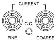
Used for fine adjustment of the current output.
