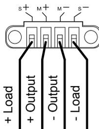
**S+, S-** Sense terminals. Connect the S+ terminal to the + positive terminal of the load. Connect the S- terminal to the - negative terminal of the load.
