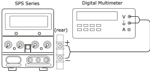
Verification step 1. Connect a multimeter as shown to the output terminals.
