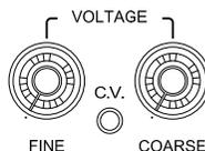
Used for fine adjustment of the voltage output.
