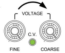
2. Turn the OVP adjuster to maximum (fully clockwise)
