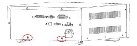
2. Fasten the 2 screws, which were removed from the step 1, with the holder 62RA-445HP101 on the rear side of unit.
