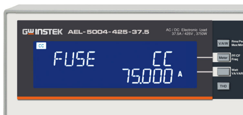
Turbo ON, Fuse Mode Test Result Screen
