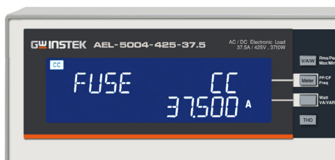
Turbo : OFF, Fuse Mode Test Result Screen
