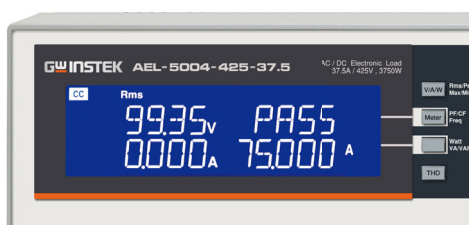
Turbo ON, Short 100 ms 75.0 A Test Result Screen
